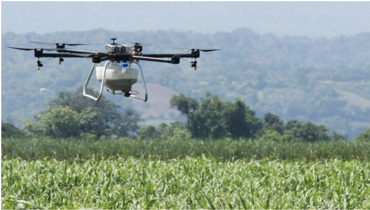
Figure 2 is an illustration of a drone spraying crops in a region of the farm where tractors and even human sprayers may fail to reach because of the crop density. Reprinted from ( Technology of Business reporter, 2018 by Chris Baraniuk )
