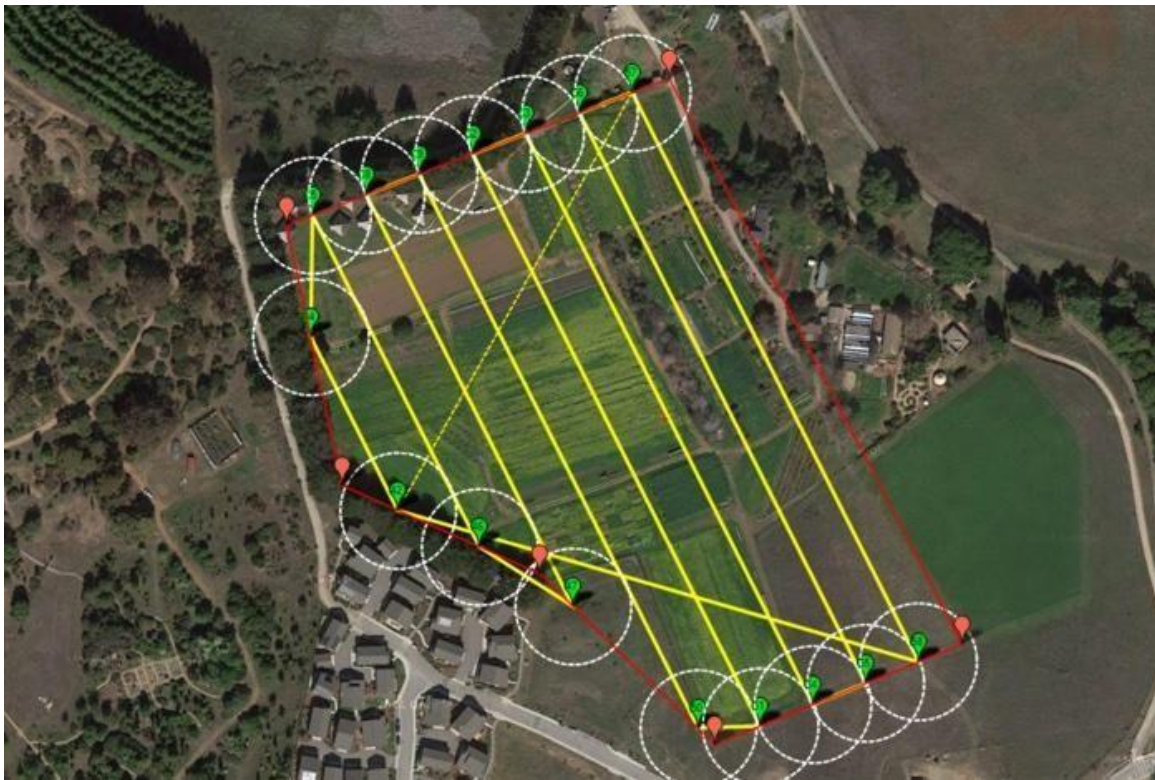
Figure 4. Picture shows flight path of unmanned aerial systems (UAS) Reprinted from ( Best Drones for Agriculture. 2019 by ANDREW NIXON )
