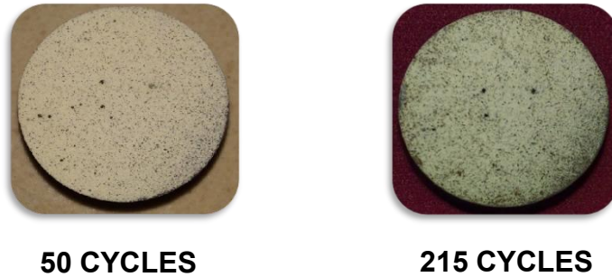
Fig 5.10: SZ3 Sample under gone Thermal Cyclic Test
