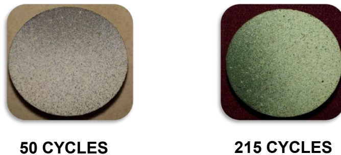
Fig 5.7: SZ2 Sample under gone Thermal Cyclic Test
