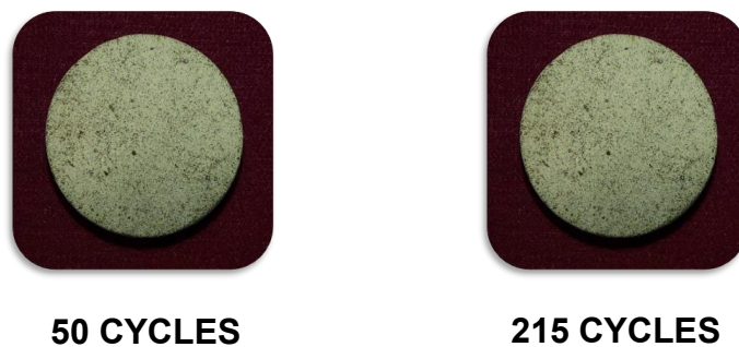
Fig 5.23: SZ3 Sample under gone Thermal Shocking Test
