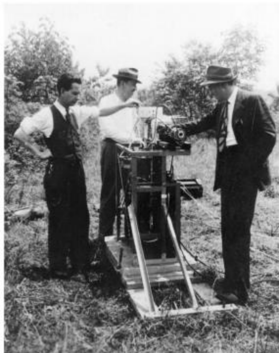
Figure 2.2: Reaction Motors, Inc. M15-G1 rocket engine being tested on the American Rocket Society's Test Stand no.2 in June 1942. [2]
