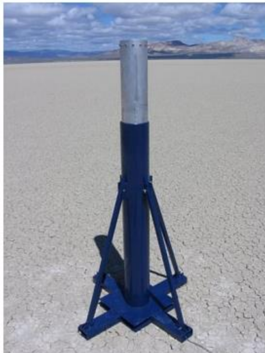
Figure 3.2: Vertical test stand with the nozzle facing upwards developed by Dewayne Doud in 2005[9]
