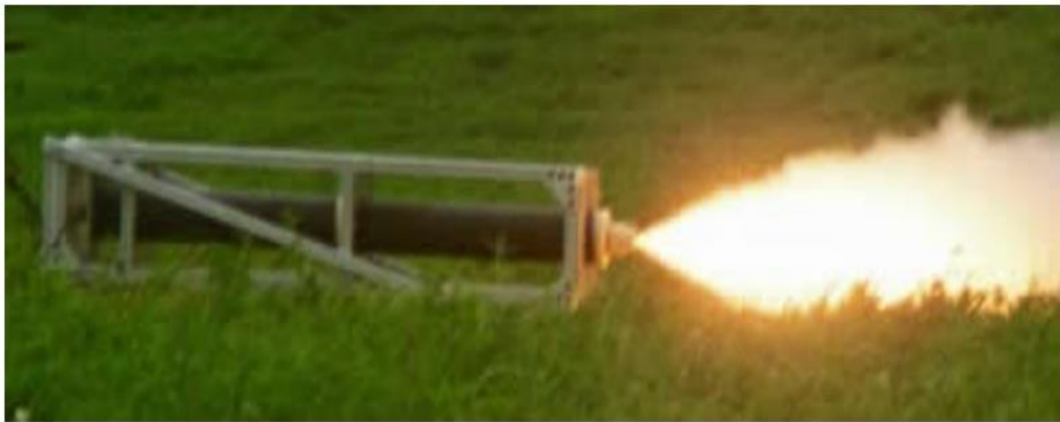
Figure 3.3: Horizontal test stand from Alexander Bruccoleri at Dartmouth College. [9]
