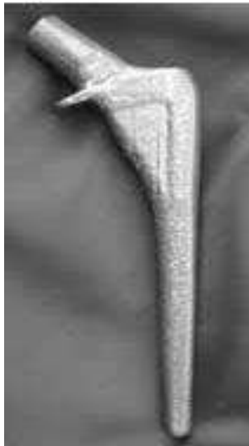
Fig 3.13: Medical LENS produced metal part Research and Development
