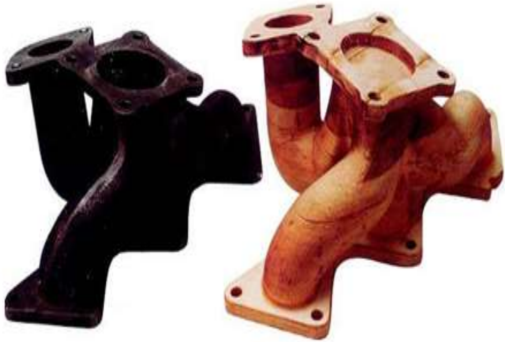
Fig 4.7: Cast metal (left) and RP pattern for sand casting
