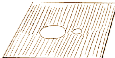
Fig 2.9: Solid ground curing process - Development of Photo mask
