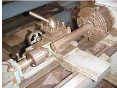
Fig. 2.24 Holding drill chuck and drill in tailstock
