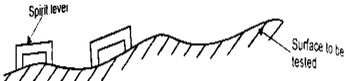
Fig:1 .1 Straightness measurement using spirit level
