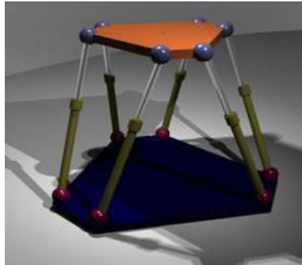
Fig: 3.3 Abstract render of a Hexapod platform (Stewart Platform)
