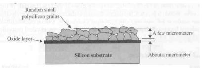
Fig. 3.12 Polysilicon deposits on a silicon substrate
