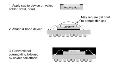
**Figure .10** Cap-on-chip packaging. Reproduced from K. Gilleo, 2001b, 'MEMS packaging issues and materials', in *Proceedings of IEEE International Symposium on Advanced Packaging: Process, Properties and Interfaces*, IEEE, Washington, DC: 1 – 5, by permission of IEEE, © 2001 IEEE
