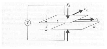
Fig2.6 Electrostatic forces in charged parallel plates
