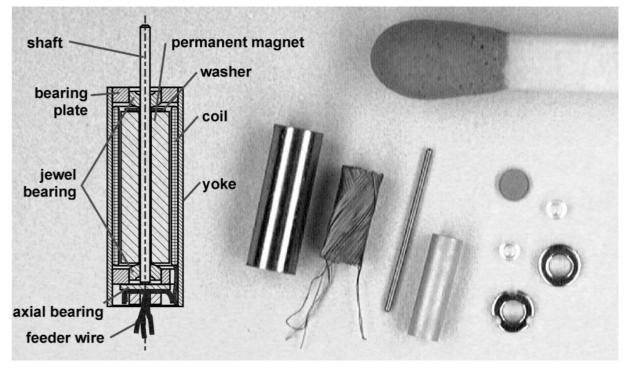
Fig-7: Construction and components of a electromagnetic micromotor
