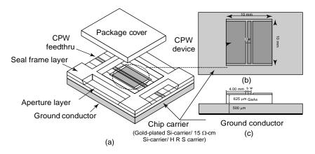
**Figure .8** (a) Typical MEMS packaging with co-planar waveguide (CPW) line; (b) top view and (c) side view Note: HRS, high-resistivity silicon. Reproduced from S.J. Kim, Y.S. Kwon and H.Y. Lee, 2000, 'Silicon MEMS Packages for coplanar MMICs', in *Proceedings of 2000 Asia-Pacific Microwave Conference, Australia, December 2000*, IEEE, Washington, DC, by per-mission of IEEE, © 2000 IEEE
