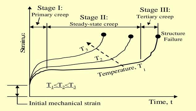
Silicon and silicon compounds have strong creep resistance. Creep is not a problem. It is the polymer materials and many solder alloys that have this problem.
