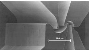
Fig.23. LIGA micro machined nozzles [Image courtesy of Wenn du Benutzer Captain Bligh,Source: Wikipedia]
