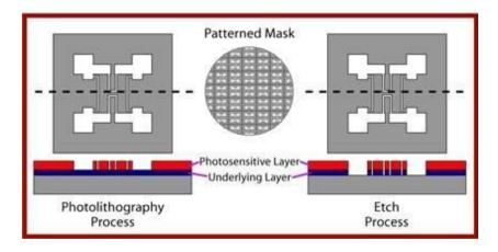
After the develop process, the exposed areas of the underlying layer are etched (removed) using either a wet or dry etch process. Once the resist pattern has been transferred to the underlying material layer, the remaining resist is removed (resist strip) leaving the patterned material layer.
