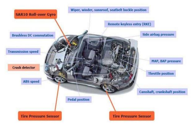
Fig-2: Typical example of microsensors used in cars
