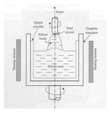
Fig 3.1 The Czochralski method for growing single crystals (Ruska [1987])
