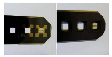
Fig .22. MEMS pressure sensor frontside (left) showing electronic sensing circuit etch in a gold film layer and backside (right) showing the chamber (look closely and you can see the beveled edges). [Images courtesy of UNM/MTTC]
