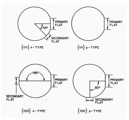
Fig.3.10 Primary and secondary flats on silicon wafers.
