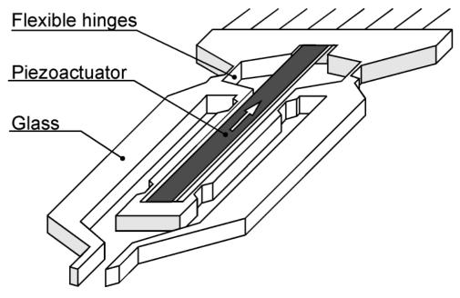
**Fig-8: MEMS microgripper**
