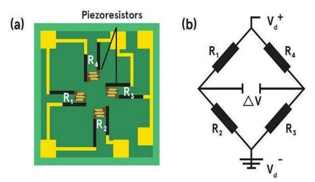
Fig-16: (a) Arrangement of Piezoresistors (b) Wheatstone bridge connection
