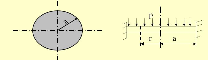
Let W = total force acting on the plate, W =  $(\pi a)p$  and m=1/V
