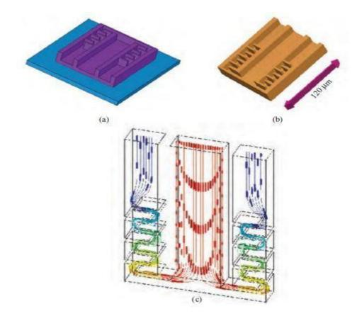
Fig-42: a)Two dimensional view of typical microfluidic channel, b) segmental view, c) Flow profile of the microfluidic channel
