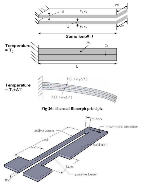
**Fig-24: Full image of thermal bimorph transducer**
