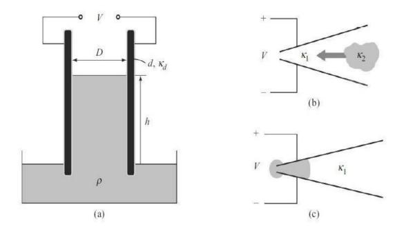
Fig-41: (a) Pellat's dielectrophoretic force experiment; (b) The dielectric liquid is attracted to regions with stronger electric field; (c) The liquid surface follows the electric field lines
