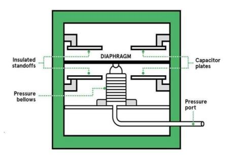
**Fig-15: Diaphragm Pressure sensor system**
