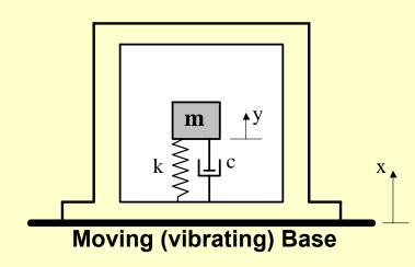
**x(t)** = the amplitude of vibration of the base
