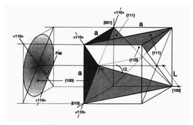
Fig. 3.11 (100) silicon wafer with reference to the unity cube and its relevant planes. (From E. Peeters, "Process Development for 3D Silicon Microstructures, with Application to Mechanical Sensor Design," KUL, Belgium, 1994.<sup>42</sup> Reprinted with permission.)
