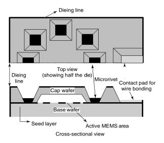
**Figure .14** View of a packaged chip using microrivets. Reproduced from B. Shivkumar and C.J. Kim, 1997, 'Microrivets for MEMS packaging: concept, fabrication and strength testing', *Journal of Microelectromechanical Systems* **6**(3): 217–225, by permission of IEEE, © 1997 IEEE
