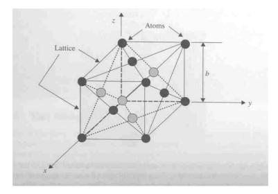
Fig 3.4 A typical face center cubic unit cell
