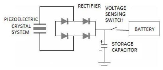
Fig-11: Piezoelectric crystal coupled with rectifier and battery for storing
