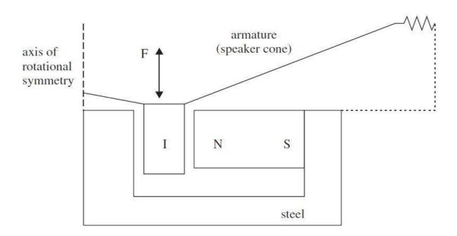
Fig-35: Typical voice coil actuator, shown driving a loudspeaker. The movable voice coil carries the current *I* and is subjected to the magnetic field from a permanent magnet with north (N) and south (S) poles.
