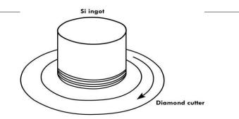
Figure 8: Inner diameter wafer slicing, used for cutting the ingots into indi- vidual wafers. The thickness is slightly higher than the final required thick- ness to account for material loss due to polishing. Adapted from Microchip fabrication - Peter van Zant.
