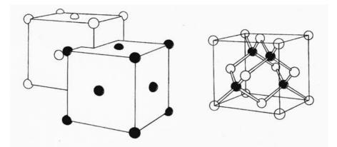
Fig 3.5 The diamond-type lattice can be constructed from two interpenetrating face-centered cubic unit cells. Si forms four covalent bonds, making tetrahedrons.
