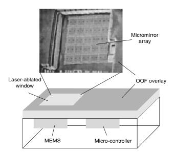
**Figure .4** COF/MEMS package of 5 5 area of micromirrors. Note: COF, chip-on-flex. Repro- duced from J.T. Butler and V.M. Bright, 2000, 'An embedded overlay concept for microsystems packaging', *IEEE Transactions on Advanced Packaging* **23**(4): 617 – 622, by permission of IEEE, © 2000 IEEE
