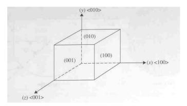
Fig 3.8 Silicon Crystal Structure and planes and Orientation
