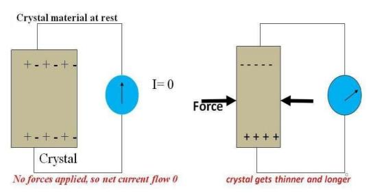
**Fig-12: Piezoelectric effect**
