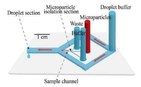
Fig-43: Typical microfluidic dispenser structure
