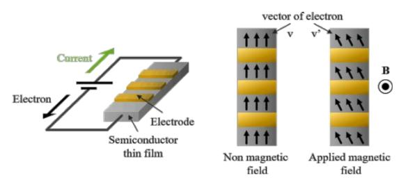
Fig-31 Magnetostrictive property using semiconductors
