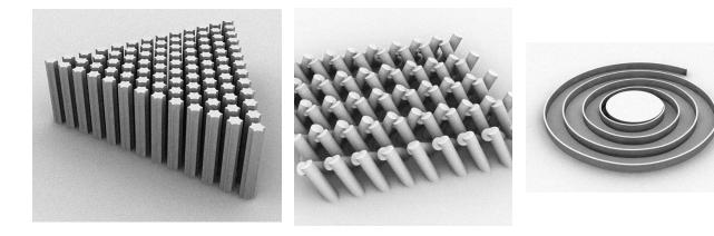
The left image represents high aspect ratio posts. Such posts can be fabricated from a LIGA mold or build into the PMMA and released. The middle image represents angled structures that can be fabricated using a LIGA process. Again, notice the high aspect ratio of the components. The right image is of a coiled spring. This would be a very difficult component to fabricate using surface or bulk micromachining. However, such components are possible with a LIGA process.
