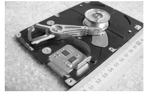
Fig-33: Typical Computer disk assembly
