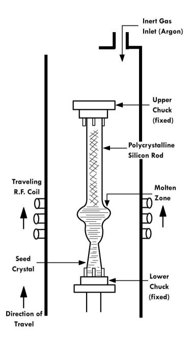
Figure 6: Schematic of the float zone technique. The polycrystalline ingot is fused with a seed crystal and locally melted by a traveling radio frequency coil. As the ingot melts and resolidifes it has the same orientation as the seed. Adapted from Microchip fabrication - Peter van Zant.
