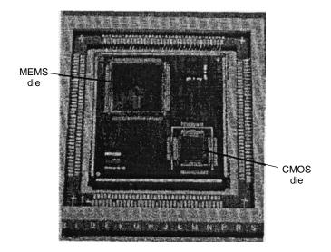
**Figure .13** MCM-D/MEMS package. Note: CMOS, complementary metal oxide semiconductor; MEMS, microelectromechanical system; MCM-D, multichip module-deposited. Reproduced from J.T. Butler, V.M. Bright and J.H. Comtios, 1997, 'Advanced multichip module packaging of micro-electromechanical systems', in *Transducers '97*, IEEE, Washington DC: 261 – 264, by permission of IEEE, © 1997 IEEE
