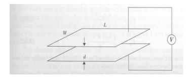
Fig 2.4 Electrically charged parallel plates
