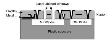
**Figure.3** Chip-on-flex MEMS packaging concept. Reproduced from J.T. Butler and V.M. Bright, 2000, 'An embedded overlay concept for microsystems packaging', *IEEE Transactions on Advanced Packaging* **23**(4): 617 – 622, by permission of IEEE, © 2000 IEEE
