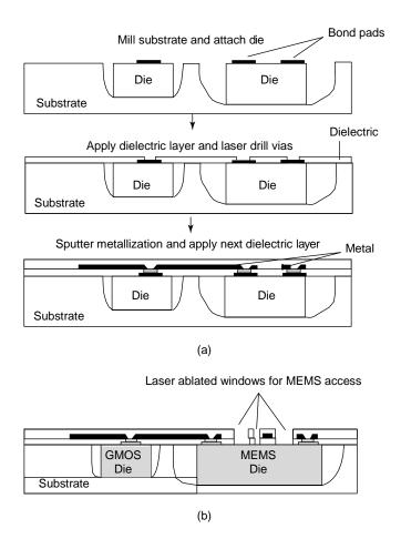
**Figure .12** (a) High-density interconnected (HDI) process; (b) MEMS access in HDI process. Reproduced from J.T. Butler, V.M. Bright, P.B. Chu and R.J. Saia, 1998, 'Adapting multichip module foundries for MEMS packaging', in *Proceedings of IEEE International Conference on Multichip Modules and High-Density Packaging*, IEEE, Washington, DC: 106 – 111, by permission of IEEE, © 1998 IEEE
