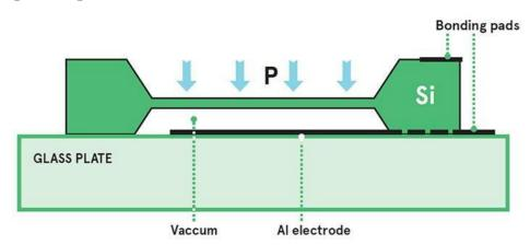
Fig-14: MEMS Capacitive pressure sensor
