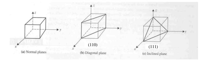
Fig 3.7 Designation of the planes of a cubic crystal
