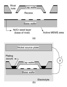
**Figure .15** Schematic diagram of (a) the prepared cap and (b) the electroplating setup. Repro- duced from B. Shivkumar and C.J. Kim, 1997, 'Microrivets for MEMS packaging: concept, fabrica- tion and strength testing', *Journal of Microelectromechanical Systems* **6**(3): 217 – 225, by permission of IEEE, © 1997 IEEE
