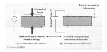
Fig 3.15 Conversion of Mechanical and electrical energies by piezoelectric crystals
