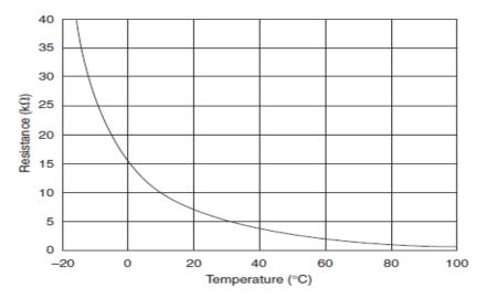
Fig-21: Temperature versus resistance response of Thermistor
