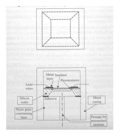
Fig 3.17 A typical packaged micro pressure sensor
