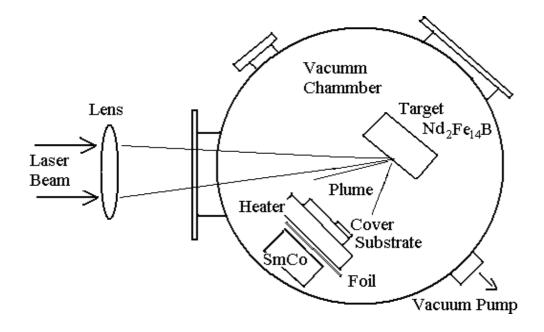
**Fig-38: Illustration of the Experiment Setup**
