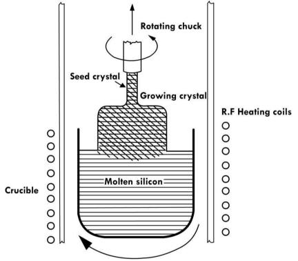
Figure 4: Schematic of the Czochralski growth technique. The polycrystalline silicon is melted and a single crystal seed is then used to nucleate a single crystal ingot. The seed crystal controls the orientation of the single crystal. Adapted from *Microchip fabrication - Peter van Zant*.
