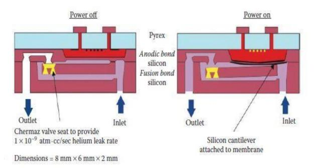
Fig-6: Examples of commercially available actuators. Thermopneumatic valves by Redwood Microsystem s (Fluistor). Normally closed shut-off microvalve featuring a liquid-filled cavity, which flexes a silicon diaphragm when heated, forcing the valve cover to lift off the valve seat.
