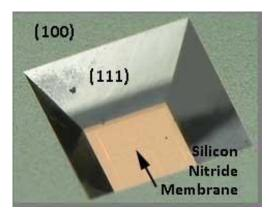
the (100) plane stops when it hits the silicon nitride which is impervious to the KOH. For the purpose of this etch, the silicon nitride layer is the etch stop layer. For the purpose of the pressure sensor, the silicon nitride serves as the membrane or diaphragm on which the sensing circuit is constructed.
