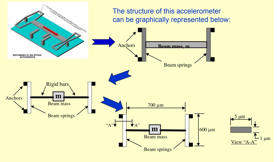
With:  $b = 10^{-6}$  m,  $B = 100x10^{-6}$  m,  $L = 600x10^{-6}$  m and  $L_b = 700x10^{-6}$  m, we have from Example 4.9 the moment of inertia of beam spring cross-section to be: I = 10.42x10<sup>-24</sup> m<sup>4</sup>
