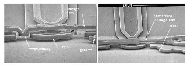
Fig 16. Without CMP (left image), With CMP (right image) [Scanning Electron Microscope (SEM) images courtesy of Sandia National Laboratories]
