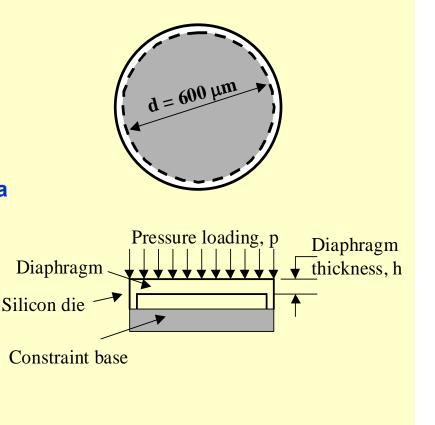
Use the condition that  $\sigma_{rr} < \sigma_{v} = 7000$  MPa and  $\sigma_{\theta\theta} < \sigma_{v} = 7000$  MPa, and
