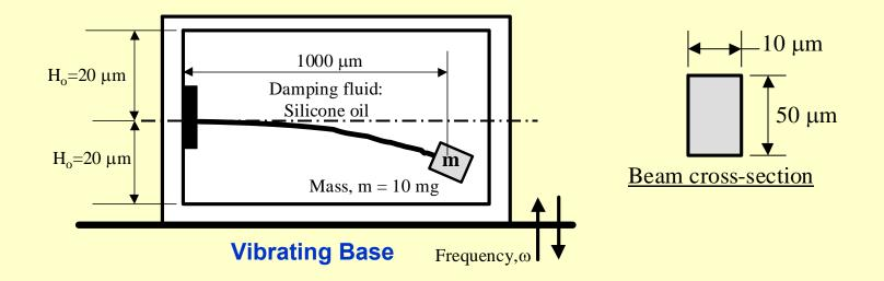
We have the beam dimensions as:  $2L = 1000 \times 10^{-6}$  m and  $2W = 10 \times 10^{-6}$  m  $\rightarrow$
