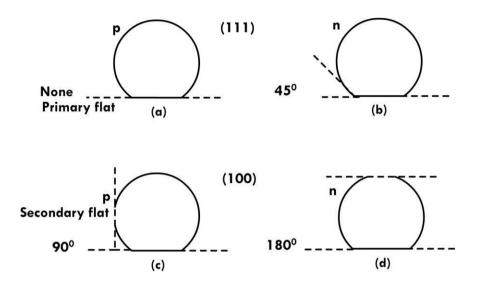
Figure 7: Flats for the different wafer types and orientations. All orientations and doping types have a primary flat, while there are different secondary flats for different types (a) p(111) (b) n(111) (c) p(100) and (d) n(100). Adapted from Microchip fabrication - Peter vanZant.
