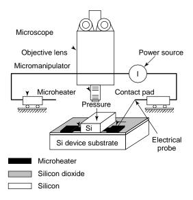
**Figure .17** Experimental setup for the localized heating and bonding test. Reproduced from L. Lin, 2000, 'MEMS post-packaging by localized heating and bonding', *IEEE Transactions on advanced Packaging* **23**(4): 608 – 616, by permission of IEEE, © 2000 IEEE
