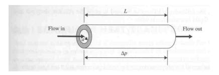
Fig 2.8 Fluid flow in a small circular conduit
