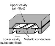
Figure .7 Self-packaged circuit constructed out of two silicon wafers. Reproduced from R.F. Dryton, 1995, *The Development and Characterization of Self-packages using Micromachining Tech-niques for High Frequency Circuit Applications*, PhD dissertation, University of Michigan, Ann Arbor, MI, by permission of the University of Michigan
