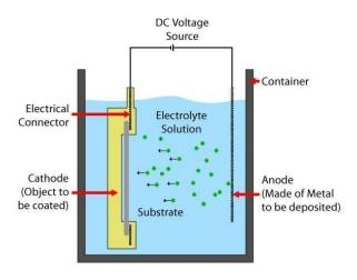
During electroplating metallic positive ions (cations) released from the anode are attracted to
