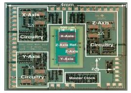
Fig. 10 Integrated 3-axes silicon micro accelerometer [Image courtesy of Sandia National Laboratories]
