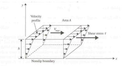
Fig .2.7 Velocity profile of a volume of moving fluid
