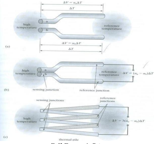
**Fig-25: Thermocouple effect**
