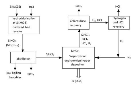
Figure 2: Schematic of the process to purify MGS to obtain EGS. The process involves conversion of silicon to trichlorosilane gas, which is purified, and then reduced to obtain silicon. Adapted from Synthesis and purification of bulk semiconductors - Barron and Smith
