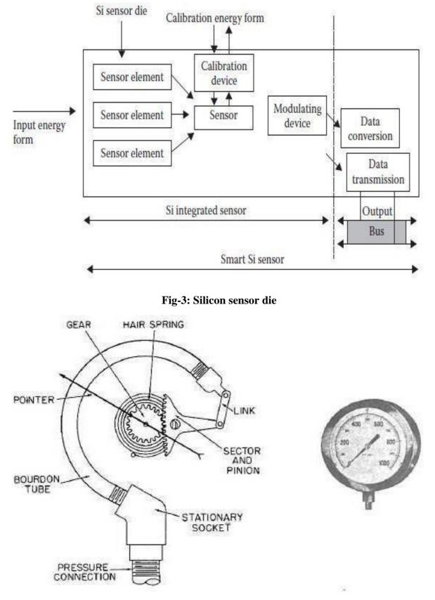
Fig-4: Example measurement system
