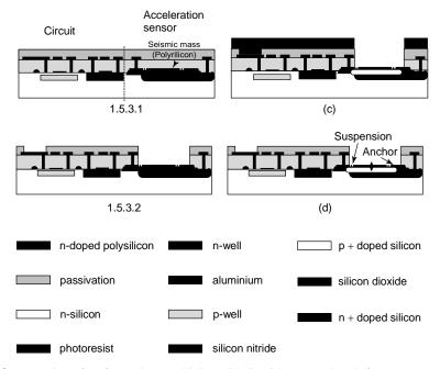
**Figure .18** Integration of surface micromachining with CMOS. Reproduced from P.J. French, 1999, 'Integration of MEMS devices', in *Proceedings of SPIE Device and Process Technologies for MEMS and Microelectroncis, Queensland Australia*, SPIE volume 3892: 39 – 48, by permission of SPIE
