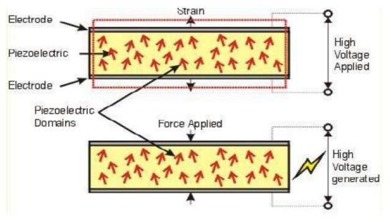
**Fig-10: Movement of charges under applied stress**
