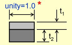
The bi-metallic strip will bend when it is subjected to a temperature rise of  $\Delta T = T - T_o$ . The strip will bend into the following shape if  $t_2 > t_1$  and  $\alpha_2 > \alpha_1$ : /
