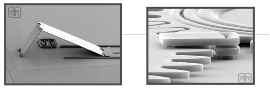
Fig.11. Pop-up Mirror (left) and geartrain with alignment pin (right) [SEM images courtesy of Sandia National Laboratories]
