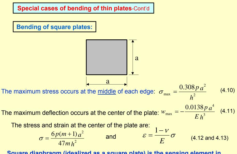
Square diaphragm (idealized as a square plate) is the sensing element in many micro pressure sensors
