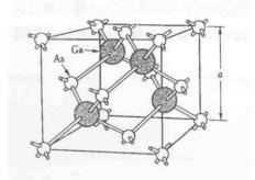
Fig 3.6 Crystal structure of GaAs
