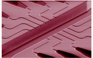
Fig.20 Microfluidic channels with high aspect ratio fluidic chambers [SEM Image courtesy of Berkeley. Ref: C. Ionescu- Zanetti, R. M. Shaw, J. Seo, Y. Jan, L. Y. Jan, and L. P. Lee (PNAS, 2005)]
