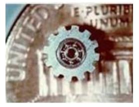
Fig. 24. This LIGA micromachined gear is used for a mini electromagnetic motor [Image courtesy of Sandia National Laboratories]
