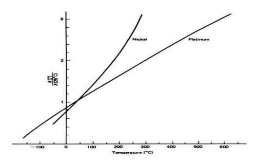
Fig-17: Temperature Vs resistance for different metals
