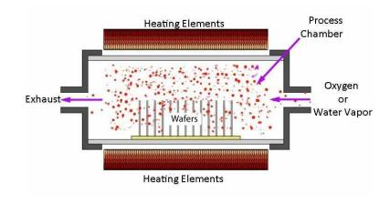
Fig.13 Diagram of an oxidation furnace's process chamber Horizontal Thermal Oxidation Furnace [Photo courtesy of University of New Mexico, Manufacturing Training and Technology Center (UNM/MTTC)]
