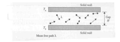
Fig 3.9 Gas flow in a micro channel
