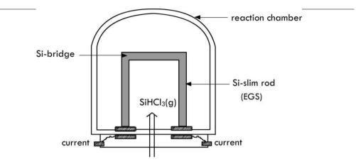
Figure 3: The Seimens deposition reactor where the purified Si is condensed. This is the electronic grade Si, same purity level as Si wafers, but polycrystalline. Adapted from Synthesis and purification of bulk semiconductors - Barron and Smith
