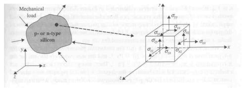
Fig 3.13 A Silicon Piezo resistance subjected to a stress field
