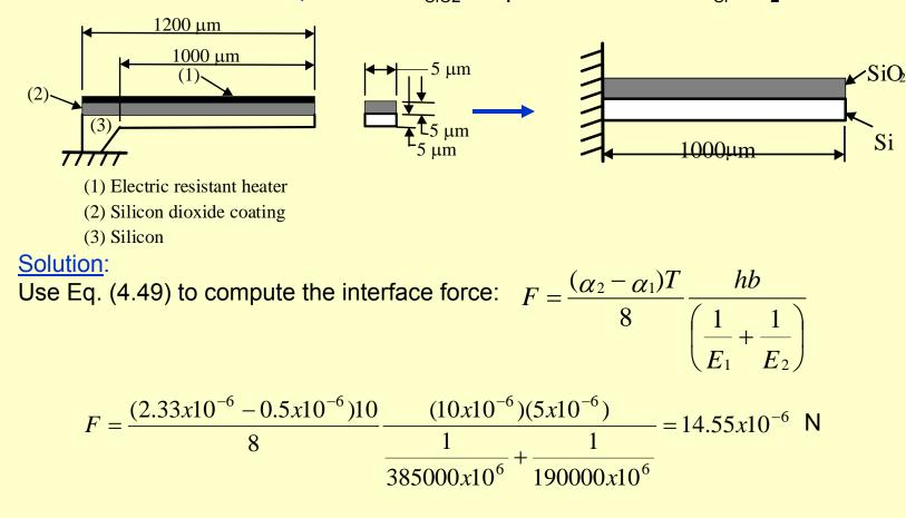
The radius of curvature of the bent beam can be computed from Eq. (4.50):
