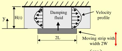
The **damping coefficient** can be found to be:  $c = 16f\left(\frac{W}{L}\right)W^3LH_o^3$ where H<sub>o</sub> = nominal thickness of the thin film.
