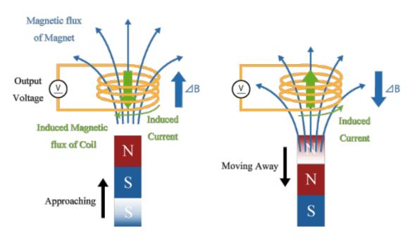
Fig-27: Principle of magnetic sensors
