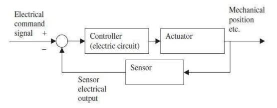
Fig-34: Basic feedback control system that may use both a magnetic actuator and a magnetic sensor.
