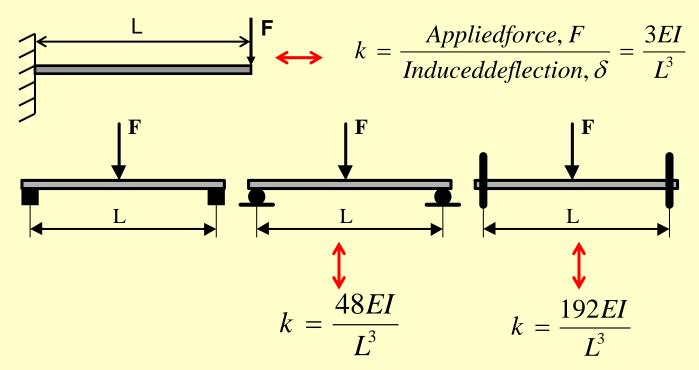
in which E = Young's modulus; I = section moment of inertia of beam cross-section.
