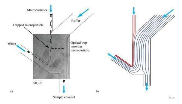
Fig-44: (a) Schematic of the microparticle isolation section, (b) Flow profile.
