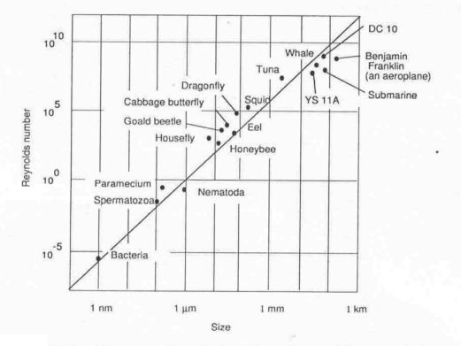
Relation between size (length) of mobile machines and Reynolds numbers of their fluid environments (adopted from Hayashi (1988)). The Reynolds number becomes around 1 when mobile machines are around 1 mm. The Reynolds number expresses the ratio between inertial force and viscous resistance. Therefore, if the machine is less than 1 mm viscous resistance dominates the dynamics. (YS 11A is a twin-engined plane.)
