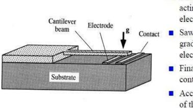
Cantilever length: 120 - 500 µm Sensitivity: 0.6 - 100 mV/g Fabrication: dry etching
