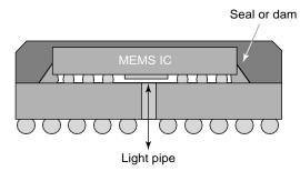
**Figure .9** Flip-chip MEMS package. Reproduced from S.J. Kim, Y.S. Kwon and H.Y. Lee, 2000, 'Silicon MEMS Packages for coplanar MMICs', in *Proceedings of 2000 Asia-Pacific Micro- wave Conference, Australia, December 2000*, IEEE, Washington, DC, by permission of IEEE, © 2000 IEEE
