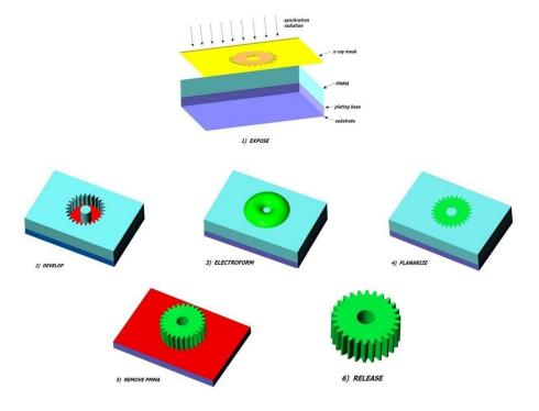
Fig. 27. [Graphic courtesy of HT MicroAnalytical, Inc.]
