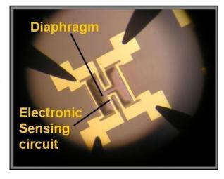
Fig. 21. [Pressure Sensor image courtesy of MTTC/UNM]
