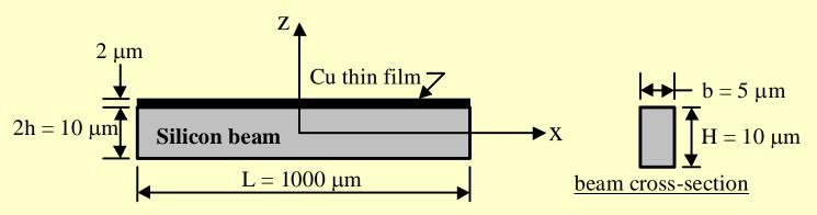
**NOTE:** This is not a bi-material strip. It is a beam made of a single material – silicon. Thermal stresses and deformations occur because of the uneven temperature distribution in beam (from top to bottom) in early stage of heating.
