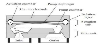
Fig-46: Cross-sectional view of a diaphragm-based micropump assembly
