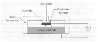
Fig 3.16 Micro sensor using polymer
