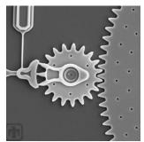
Fig. 10 These gears are very thin, 2 to 3 microns in thickness (or height), but can be hundreds of microns wide. Each gear tooth is smaller than the diameter of a red blood cell (8 to 10 microns). These gears rotate above the surface of the substrate. [SEM courtesy of Sandia National Laboratories]
