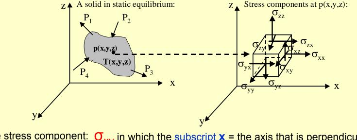
The stress component:  $O_{xy}$  in which the subscript **x** = the axis that is perpendicular to the plane of action. The subscript **y** = the direction of the stress component.
