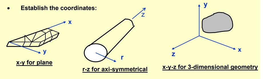
(2) Develop FE mesh (i.e. discretizing the structure):
