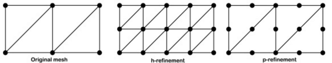
**h-method** → The h-method improves results by using a finer mesh of the same type of element. This method refers to decreasing the characteristic length ( $h$ ) of elements, dividing each existing element into two or more elements without changing the type of elements used.
