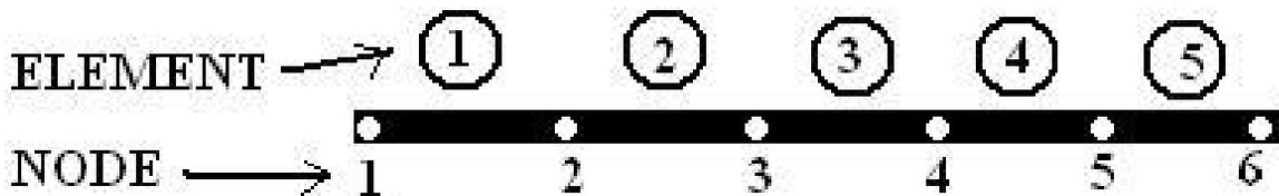
As shown in the figure, a one dimensional structure is divided into several elements and the each element has 2 nodes.
