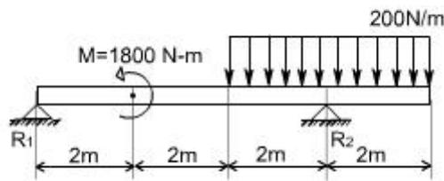
Fig.5.39 Overhanging beam with different loads
