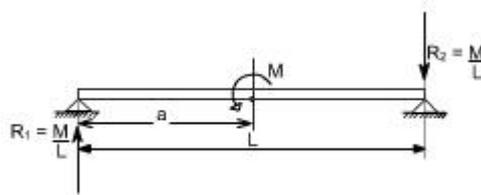
Fig.5.37 SSB with force and Couple
