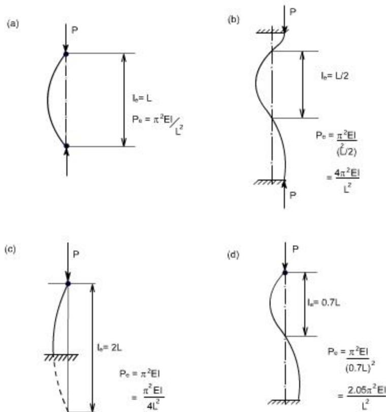
Fig. 5.8 Different End conditions loading
