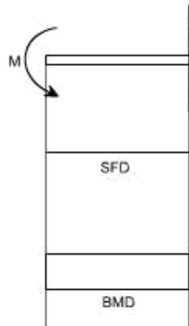
Fig. 3.24 Pure bending State for Cantilever
