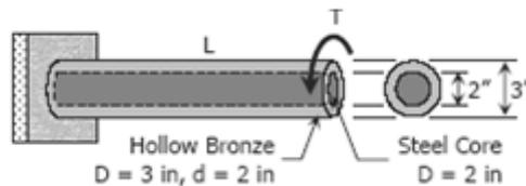
Fig. 4.13 Composite shaft
