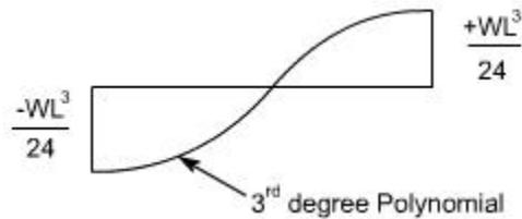
Fig. 5.19 SSB with UDL Deflection and Slope
