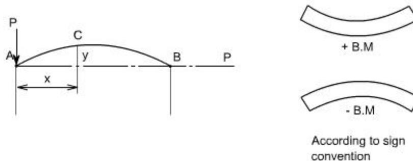
Fig. 5.3 Strut with Pinned Ends sign convention
