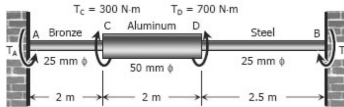
Fig. 4.11 Stress developed in each segment with respect to  $T_A$
