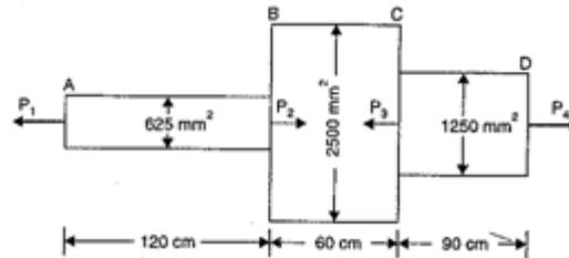
Fig. 1.8 Bar with varied cross section and Axial loads
