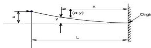
Fig. 5.5 One End fixed and other is free End condition
