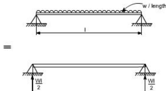
Fig. 5.17 SSB with UDL
