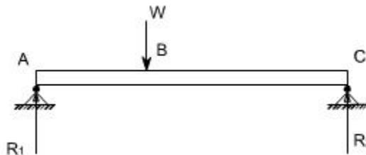
Fig.5.22 SSB with a point load reaction marked diagram
