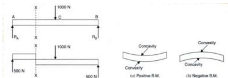
Fig. 3.12 Shear force and Bending Moment Sign Convention
