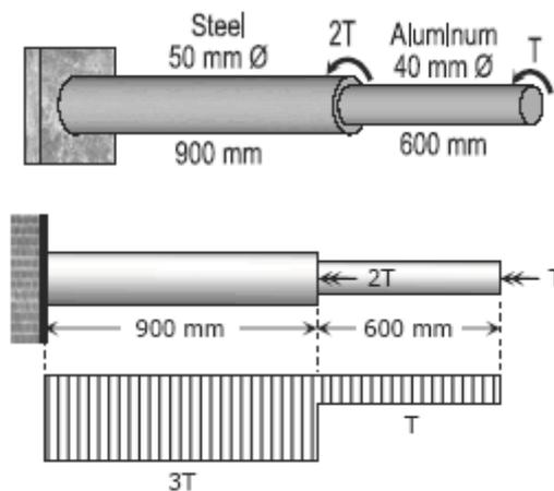
Fig. 4.7 Stepped shaft with Torque applied
