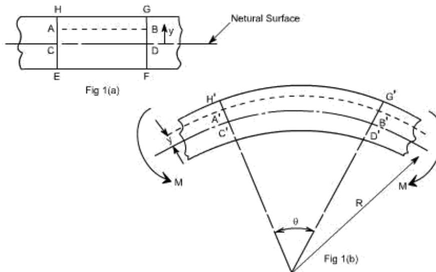
Fig. 3.21 Before and after Bending to an arc
