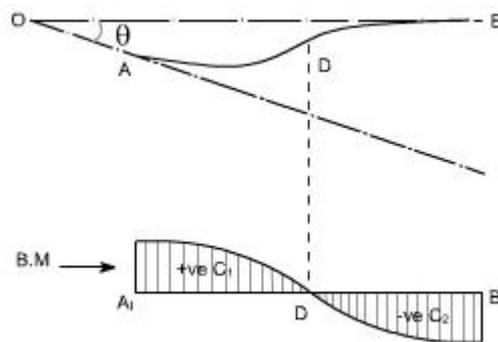
Fig.5.27 Contraflexure point
