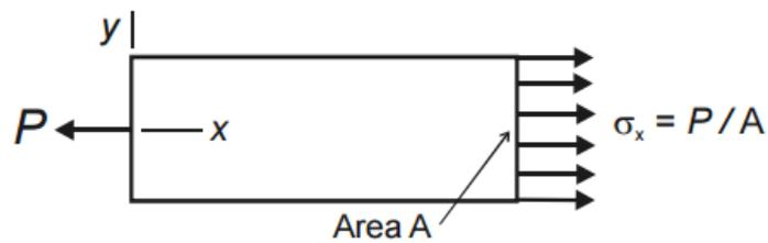
Fig. 2.20 ‘2D’ view of Normal section
