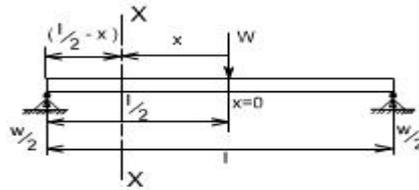
Fig.5.23 SSB with a Mid-point load
