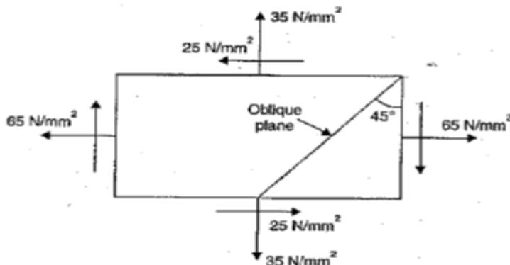
Fig. 2.11 Rectangular bar Stress state
