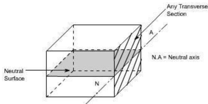
Fig. 3.25 Position of Neutral Surface/Axis
