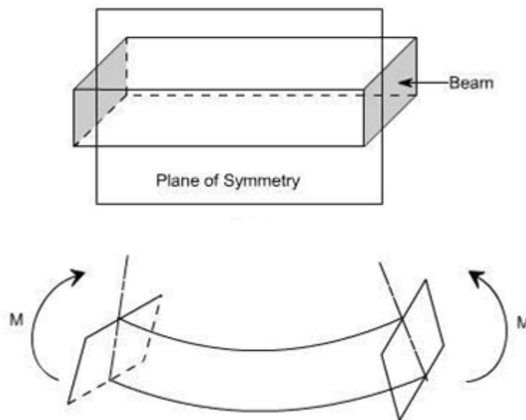
Fig.3.22 Plane of Bending
