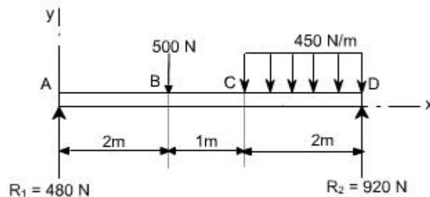
Fig.5.32 SSB with different loads
