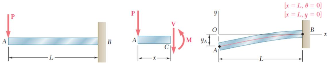
Fig. 5.10 Cantilever beam subjected to a point load and reactions
