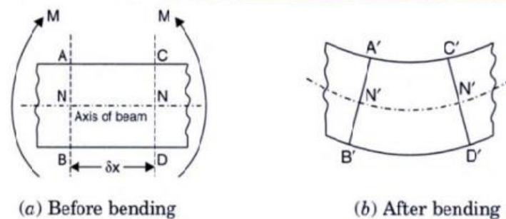
Fig. 3.20 Before and after Bending of Beam
