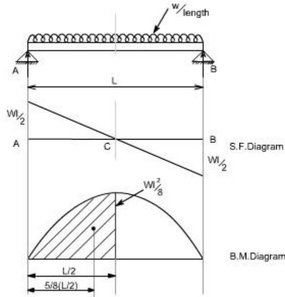
Fig.5.30 SSB with UDL – SF & BM diagram
