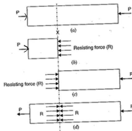
Fig. 1.2 Stress distributions during compression
