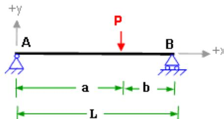
Fig. 3.9 Concentrated or point load
