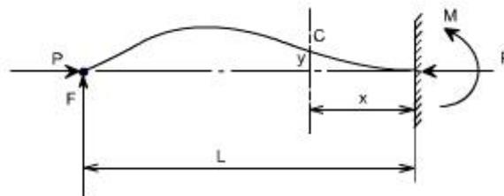
Fig. 5.7 One end Fixed and oer pinned End conditions
