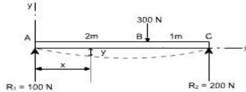
Fig.5.34 SSB with point load
