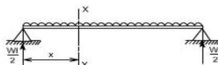
Fig. 5.18 SSB with UDL a section at X-X
