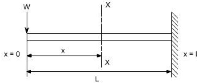
Fig. 5.15 Cantilever Beam with Concentrated Load at the free end
