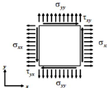
**Fig. 2.14 Element of a structure showing a biaxial stress system**
