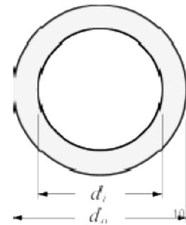
Fig. 4.3 Hollow Shaft
