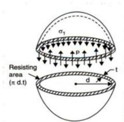
**Fig. 2.17 Spherical shell**
