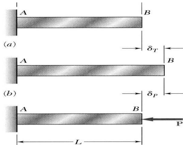
Fig. 1.10 Thermal expansion and contraction
