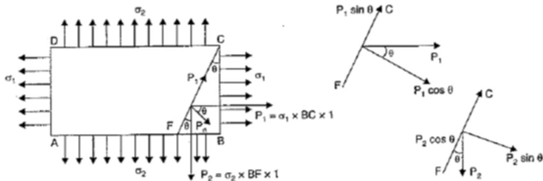
Fig. 2.3 Member subjected to Direct stress in two perpendicular directions
