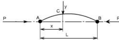
Fig. 5.2 Strut with Pinned Ends
