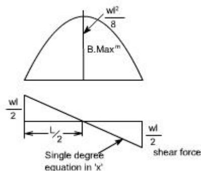
Fig. 5.20 SSB with UDL SF & BM
