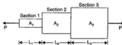
Fig. 1.5 Bar with varied cross sections and Axial load
