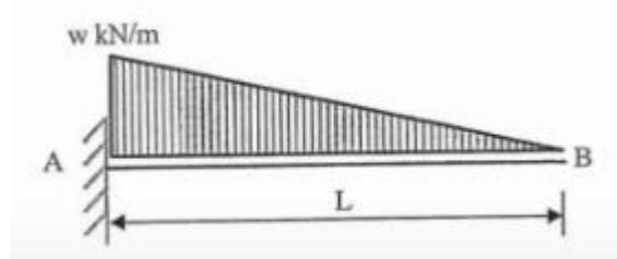
Fig. 3.11 Uniformly varying load
