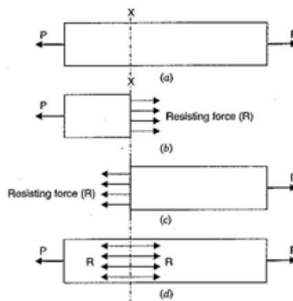
Fig. 1.1 Stress distributions during Tension
