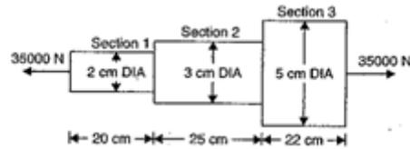
Fig. 1.6 Bar with varied cross sections and Axial load as 35000N
