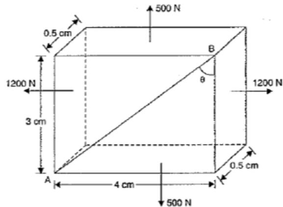
Fig. 2.4 Cube at loading condition
