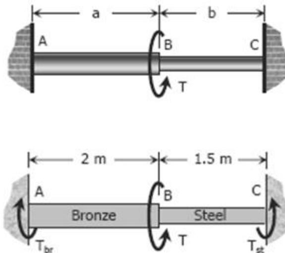
Fig. 4.8 Stepped shaft with Torque
