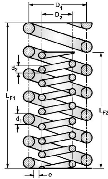
Fig.4.22 Helical Spring in parallel
