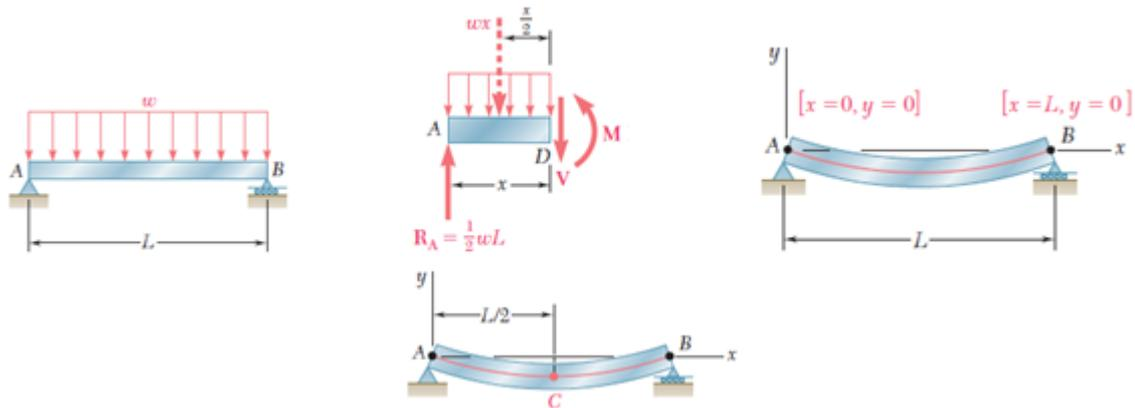
Fig. 5.11 Simply supported beam subjected to UDL
