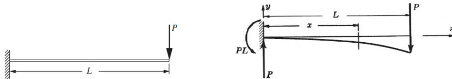
Fig. 5.9 Cantilever beam subjected to a point load at free end.
