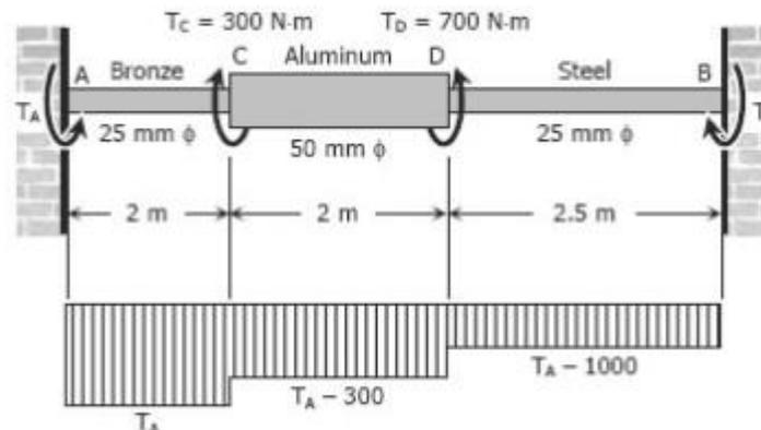
Fig. 4.12 Stress developed in each segment
