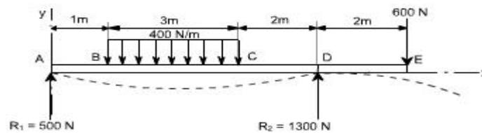
Fig.5.35 Overhanging Beam with different loads
