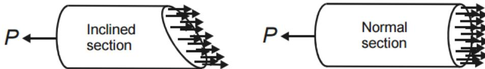
Fig. 2.19 Normal and Shear stresses pattern
