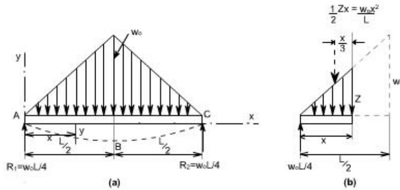
Fig.5.36 SSB with Triangular load
