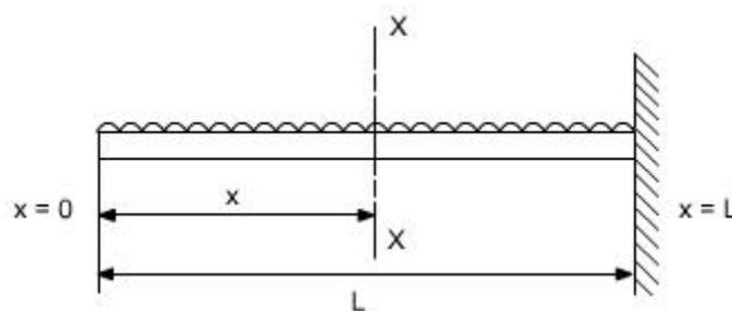
Fig. 5.16 Cantilever Beam with UDL
