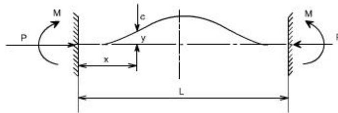
Fig. 5.6 Both Ends in fixed End condition
