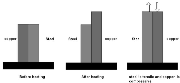
Fig. 1.11 Thermal expansion on Composite bar
