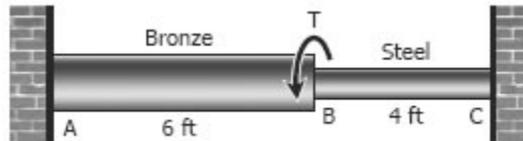
Fig. 4.9 Shaft with Torque applied
