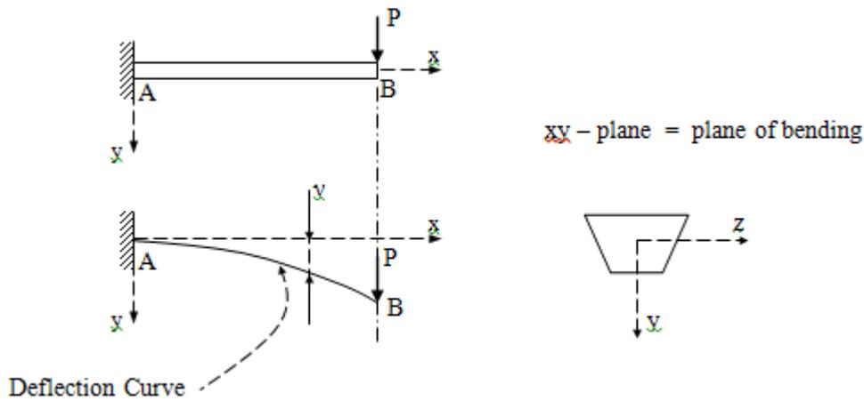
Fig. 3.27 Cantilever Beam with a point load at free end
