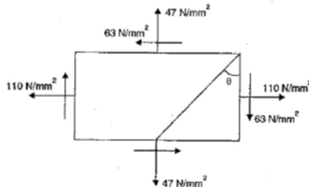
Fig. 2.7 Stress acting on Rectangular block
