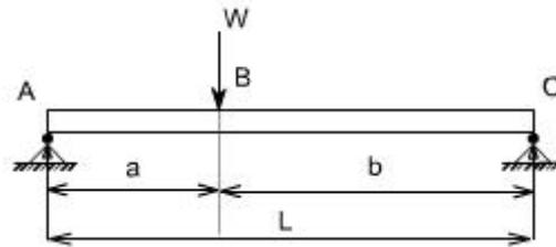
Fig.5.21 SSB with a point load acting elsewhere in the beam
