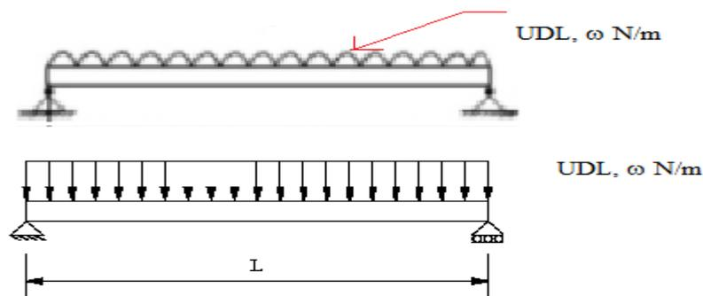
Fig. 3.10 Uniformly distributed load
