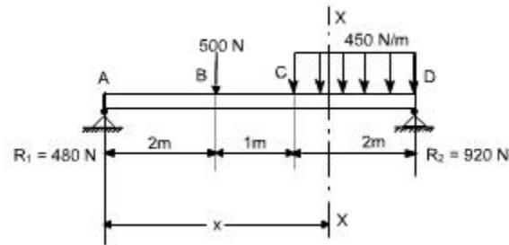
Fig.5.31 SSB with different load intensities
