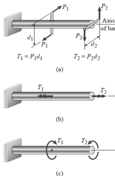
Fig. 4.1 Shaft subjected to Torsion
