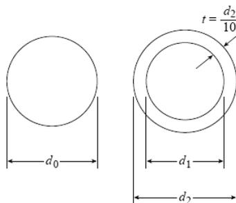
Fig. 4.4 Solid and Hollow shaft
