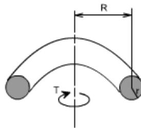
Fig.4.17 Helical Spring wire under Torque ‘T’
