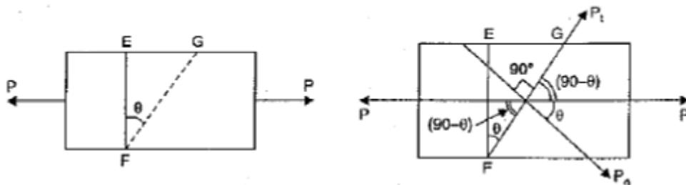
Fig. 2.1 Direct Stress in one plane
