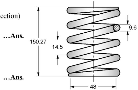
Fig.4.21 Helical Spring
