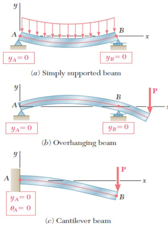
Fig. 5.13 SSB with UDL
