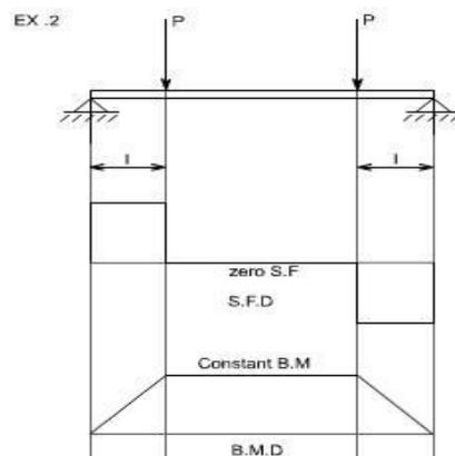
Fig. 3.23 Pure bending State for SSB
