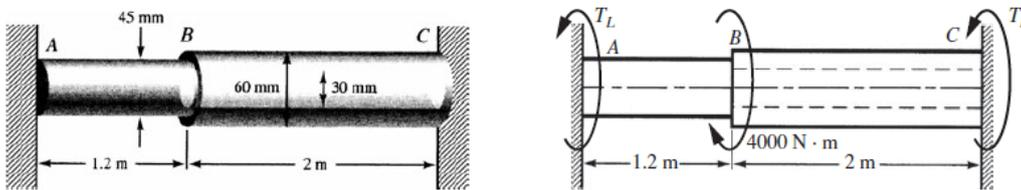
Fig. 4.5 Stepped shaft subjected to Torque
