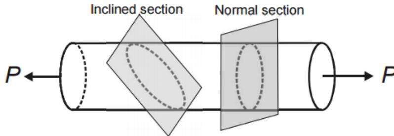
Fig. 2.18 Normal and Shear stresses on inclined planes
