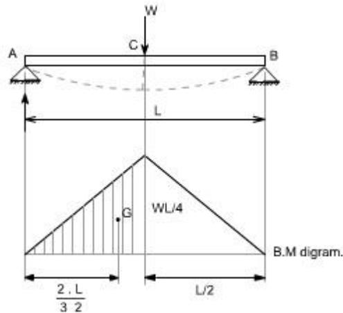
Fig.5.29 SSB and Mid-point Load - BM diagram
