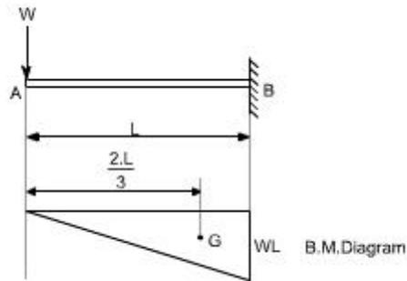
Fig.5.28 Cantilever point load at free end BM diagram
