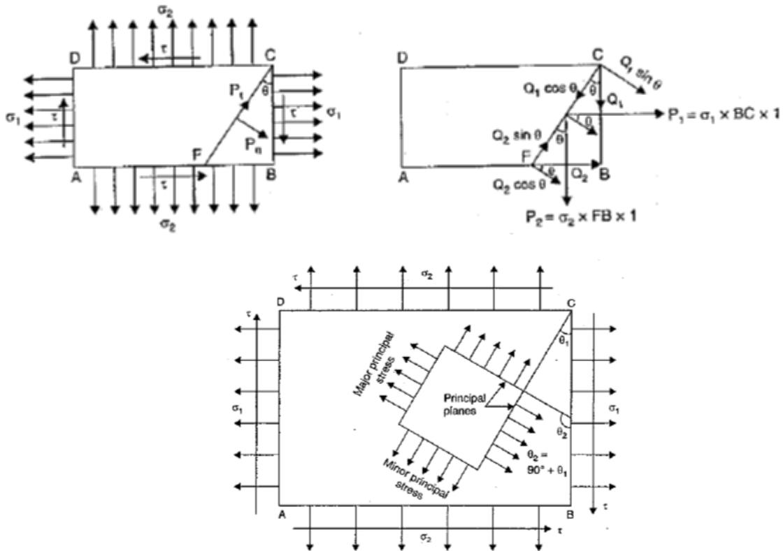
Fig. 2.5 Principal Planes Identification diagram
