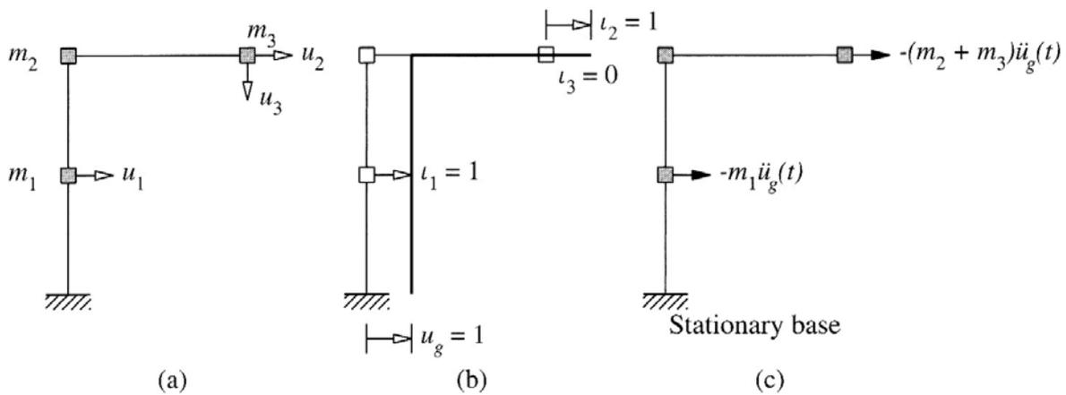
**Figure 9.4.4** (a) L-shaped frame; (b) influence vector  $\mathbf{v}$ : static displacements due to  $u_g = 1$ ; (c) effective earthquake forces.
