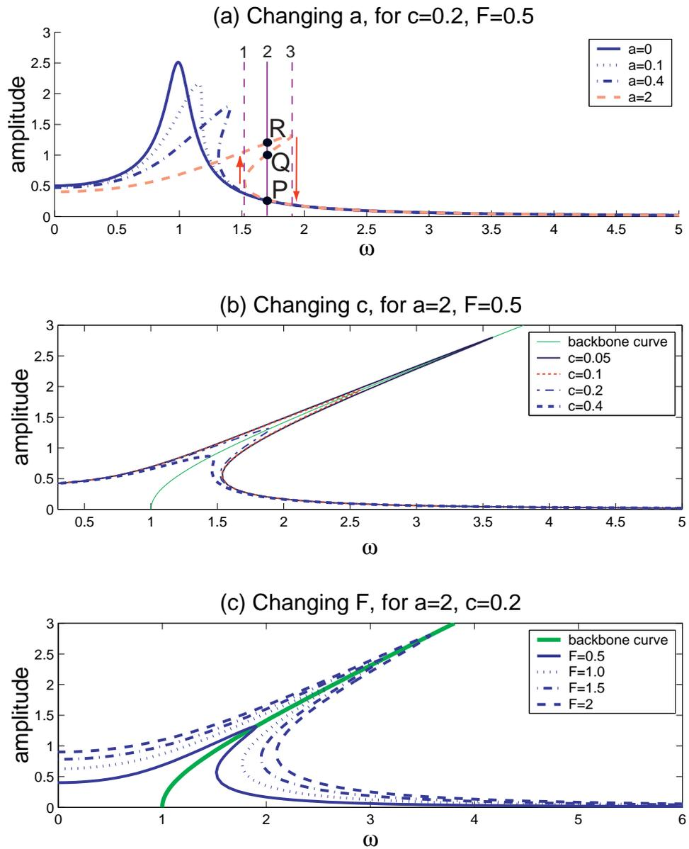
Figure 4: Forced vibrations of a nonlinear system, via harmonic balance. See text for details.
