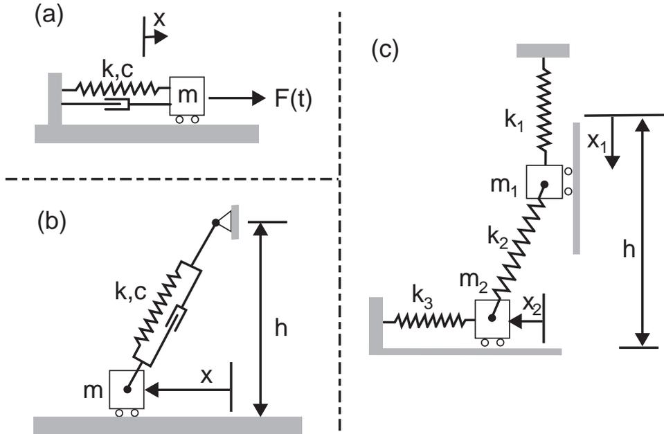
Figure 2: (a) A linear, damped, forced system. (b) A nonlinear system. The spring has a free length  $L_0 > h$ . (c) A nonlinear two degree of freedom system. Mass  $m_1$  is constrained to move frictionlessly in the vertical direction, while mass  $m_2$  moves in the horizontal direction. Gravity is neglected, for simplicity.
