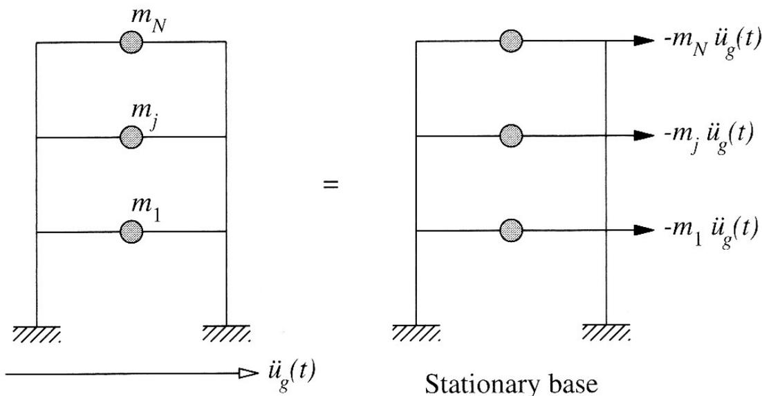
**Figure 9.4.2** Effective earthquake forces.
