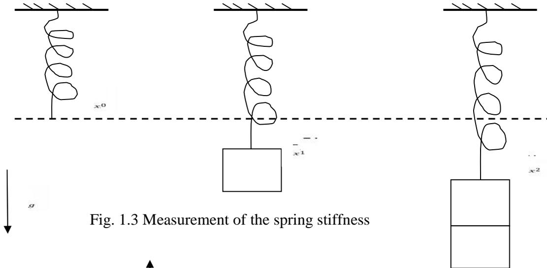
Fig. 1.3 Measurement of the spring stiffness
