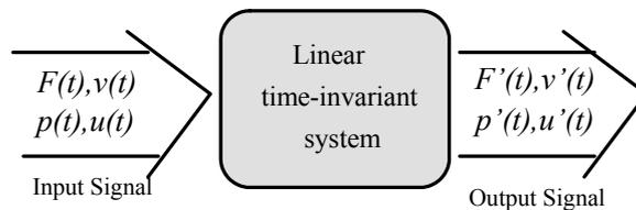
Fig. 0-1 A linear time-invariant system describes the relationship between an input signal and an output signal. For example, the input signal could be a velocity  $v(t)$ , and the output signal a force  $F(t)$ , or the input signal an acoustic pressure  $p(t)$  and the output signal an acoustic particle velocity  $u'(t)$ . [Sound and vibration book by KTH[1]]
