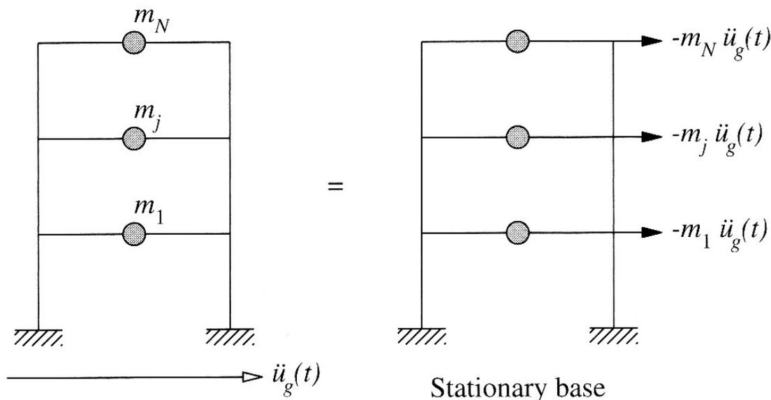
**Figure 9.4.2** Effective earthquake forces.
