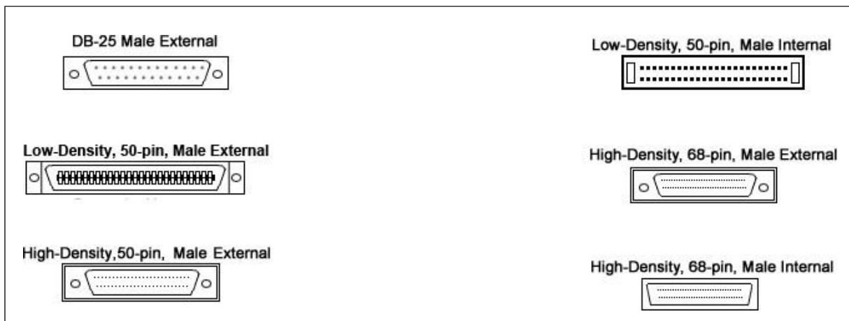
Fig No.29 commonly-used SCSI connectors on computers and devices
