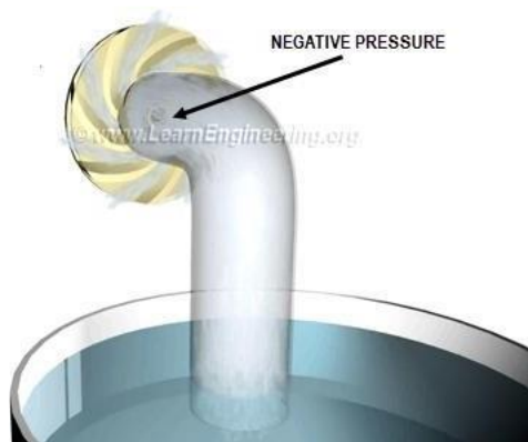
Fig.2 Negative pressure created by displacement of water from the eye helps to suck fresh stream of water
