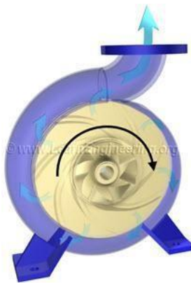
Fig.3 Water which leaves the impeller gets collected inside the casing, flow direction is also marked
