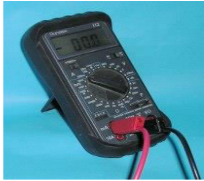
Fig. 5: Digital multimeter where the current range is selected.
