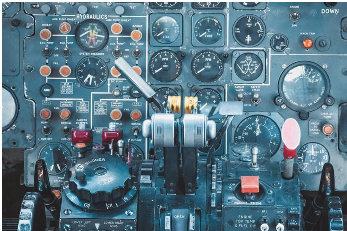
Fig. A pilot's cockpit filled with flight instruments such as altimeters and fuel levels
