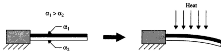
Figure 17. Thermal actuation of dissimilar materials
