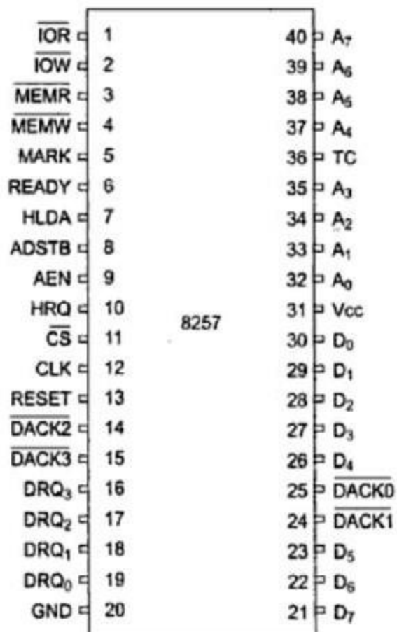
Fig 3.30 Pin Description of 8257
