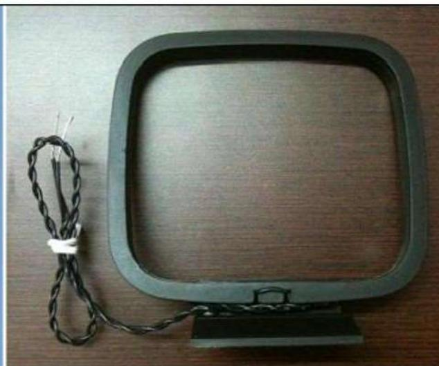
Fig 2: Square loop antenna
