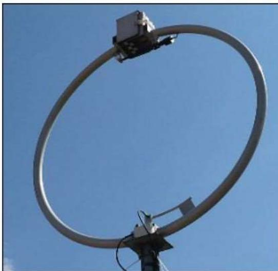
Fig 1: Circular loop antenna
