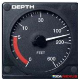
Analogue display – easy to read at a glance, often uses colour to communicate information but not as accurate as the digital equivalent.
