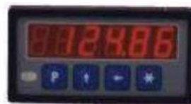
Digital display – very accurate, but can be difficult to read at a glance especially when figures change quickly.
