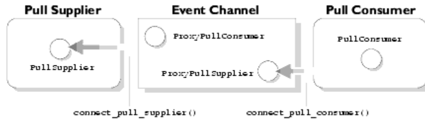
Figure 3.17: Pull Supplier and Pull Consumer Connecting to an Event Channel in the Untyped Model
