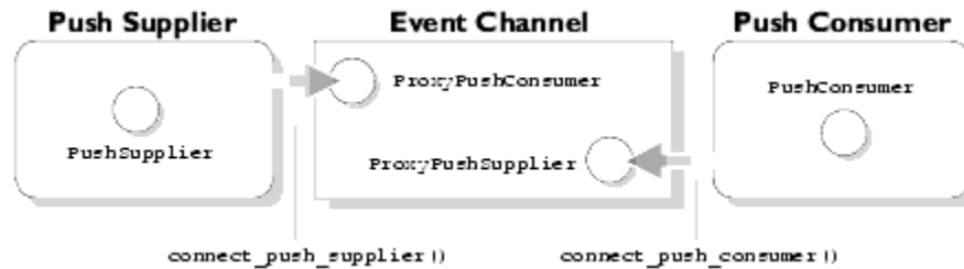
Figure 3.16: Push Supplier and Push Consumer Connecting to an Event Channel in the Untyped Model
