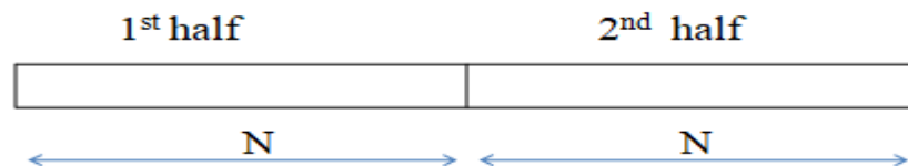
Fig. 1.7. An input buffer in two halves.
