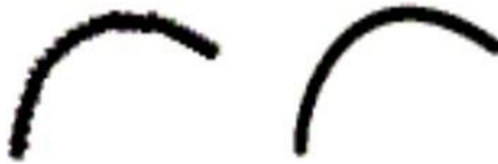
Fig 1.11. The image on the right shows the result of anti-aliasing through the use of higher resolution.
