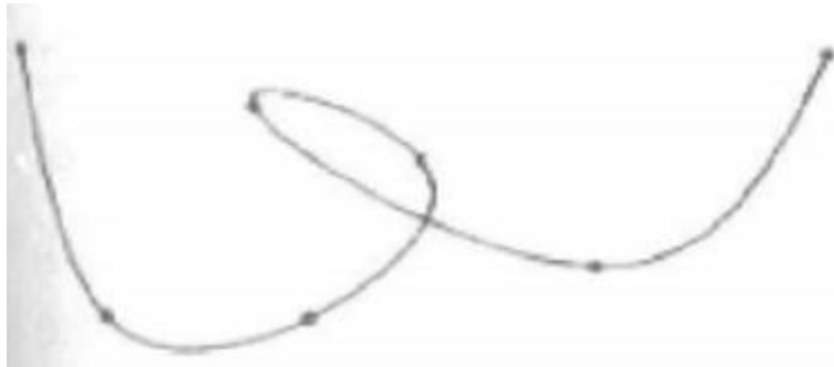
Fig. 3.13 Control Points (indicated by dots) govern the shape of the Curve
