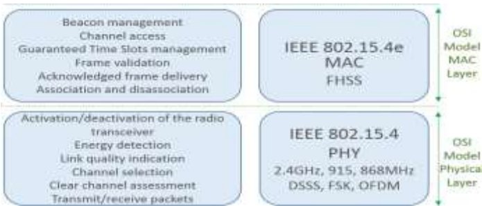
Figure 3.10 IEEE 802.15.4 compared with OSI reference model.
