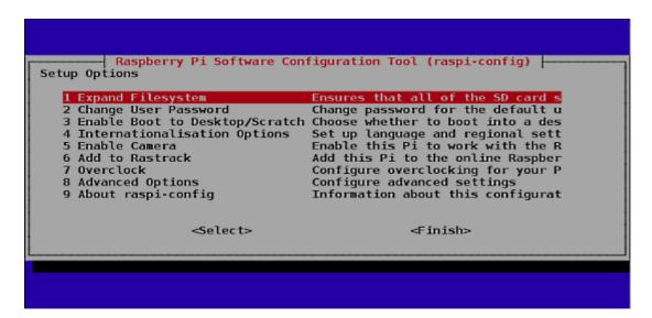
Fig. 6 Raspberry Configuration
