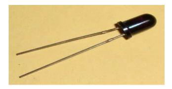
Fig. 5 Photo diode
