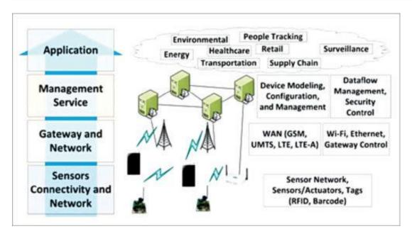
Fig. 2 IoT Architecture Layers
