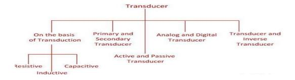
Fig. 1 Types of Transducer
