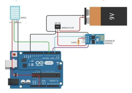
Fig. 6 Circuit diagram for monitoring Humidity and Temperature in IOT cloud
