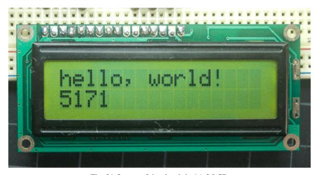
Fig. 21 Output of the sketch in 16x2 LCD
