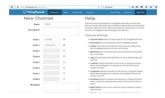
Fig.7 Creating new channel on ThingSpeak cloud
