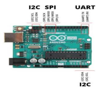
Fig.7 Arduino with I2C and SPI
