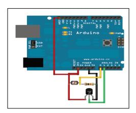
Fig 27 Temperature Sensor
