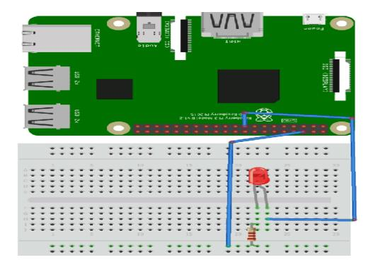
Fig 19 LED with Raspberry pi
