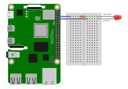
Fig. 16 Raspberry pi with LED
