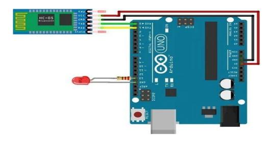
Fig. 5 Arduino with Bluetooth Connection
