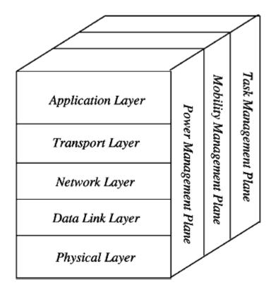
Fig. 27 Wireless Sensor Network Architecture
