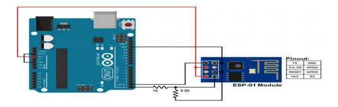
Fig. 4 ESP8266 (ESP-01) Module with Arduino UNO board
