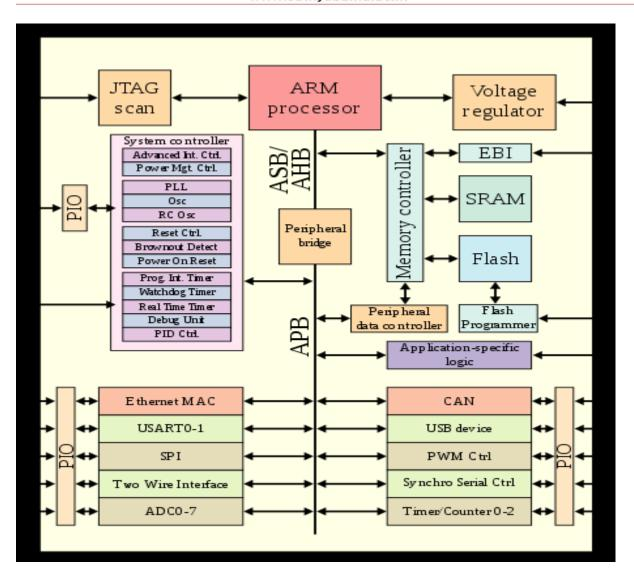
Fig. 3 Microprocessor-based system on a chip
