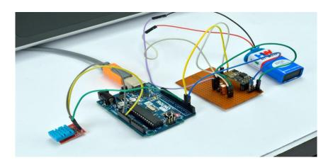
Fig. 5 Arduino with DHT sensor
