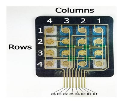
Fig. 24 keypad Structure
