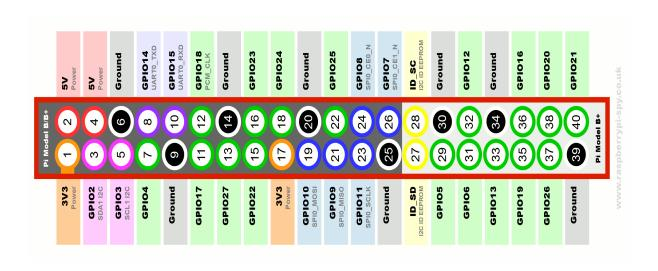
Fig. 9 GPIO Pins
