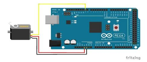
Fig. 11 Arduino with Servo motor
