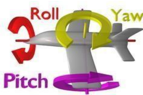
Fig 1.9: Attitude degrees of freedom for an airplane.
