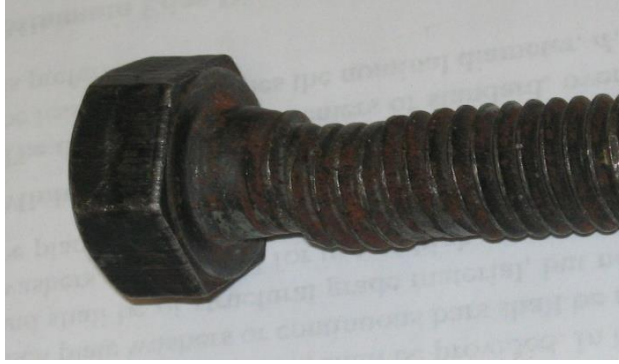
FAILURE OF BOLT IN DOUBLE SHEAR
