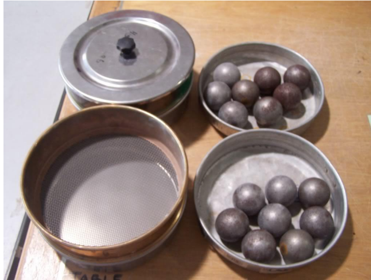
FIG.9 LOS ANGELES ABRASION TEST ON AGGREGATE
