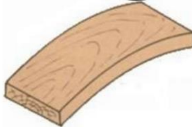
FIG.11 BOWING OF WOOD BY FAULT SEASONING
