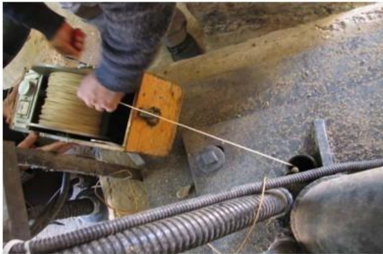
Measuring water level by M-scope
