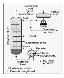
Distillation columns are used in a very broad range of applications. In sugar industries, the distillation of a mixture of water and different alcohols, produced by fermentation of sugar. Pure oxygen, used for medical purposes is produced by the distillation process. Oil refineries make use of distillation for separating all the petroleum by products.
