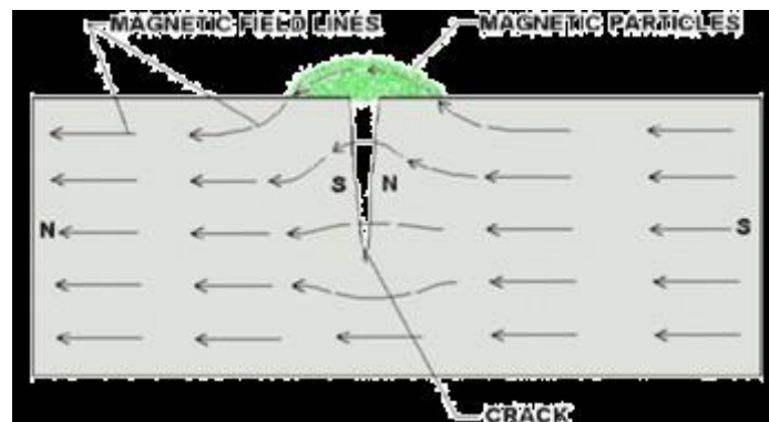
Figure - Principle of Magnetic particles Inspection
