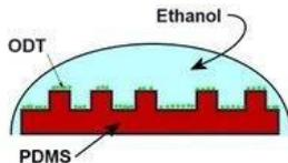
ODT from the solution settles down onto the PDMS stamp. Stamp now has ODT attached to it which acts as the ink.
