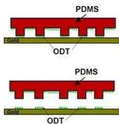
The PDMS stamp with the ODT is placed on the gold substrate. When the stamp is removed, the ODT in contact with the gold stays stuck to the gold. Thus the pattern from the stamp is transferred to the gold via the ODT "ink."
