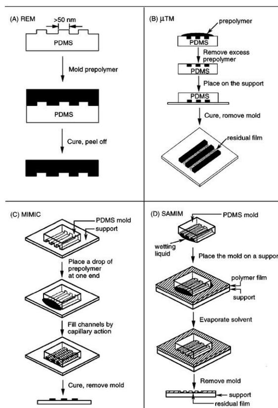
**Figure** Schematic illustration of procedures for (a) replica molding (REM), (b) microtransfer molding ( $\mu$ TM), (c) micromolding in capillaries (MIMIC), and (d) solvent-assisted micromolding (SAMIM).
