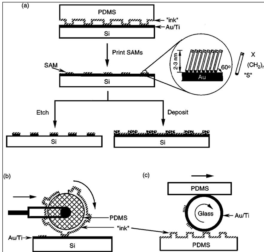
**Figure** Schematic procedures for  $1uCP$  of hexadecanethiol (HDT) on the surface of gold: (a) printing on a planar surface with a planar stamp (b) printing on a planar surface over large areas with a rolling stamp, and (c) printing on a nonplanar surface with a planar stamp.
