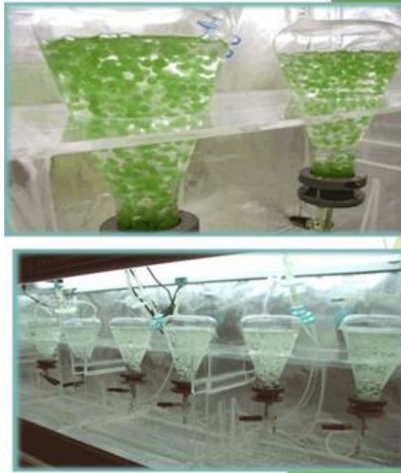
Figure 2.14: Immobilized algae used in bioreactor
