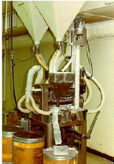
Figure :13 Tablet press with load hopper and spiral dust pickups for product recovery
