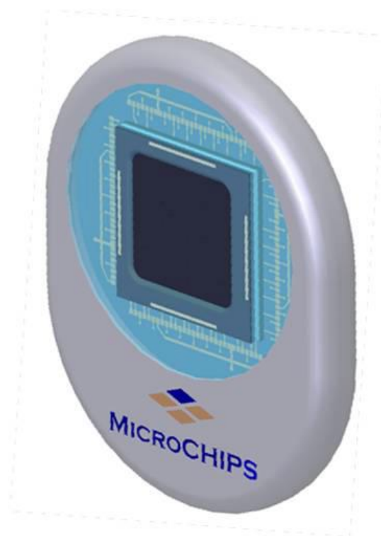
Fig-25: MicroCHIPS Subcutaneous Active Drug Delivery System
