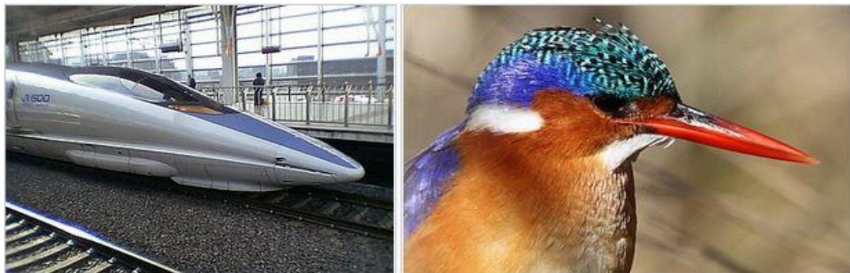
Fig-1: (b) The streamlined design of Shinkansen 500 Series (left) mimics the beak of kingfisher (right) to improve aerodynamics.
