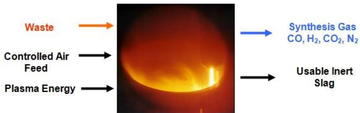
Figure 1: Plasma gasification process flow chart
