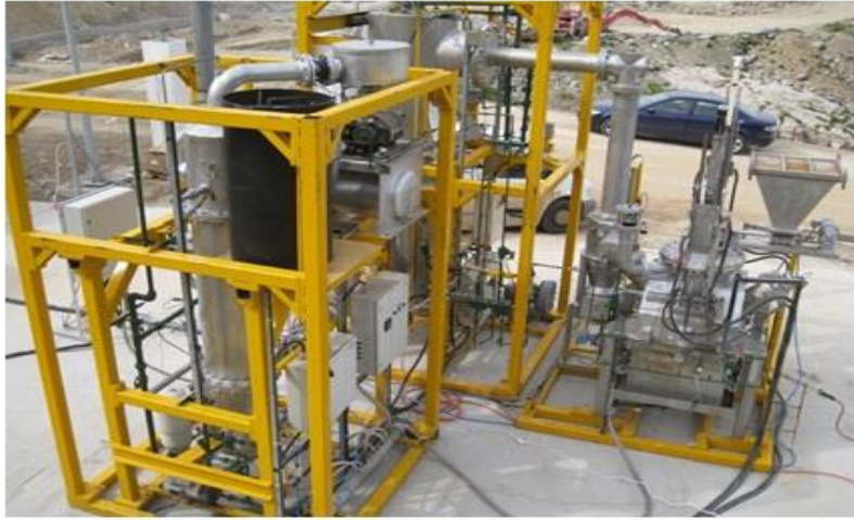
Figure 3: Another General view of the demonstration gasification / vitrification unit
