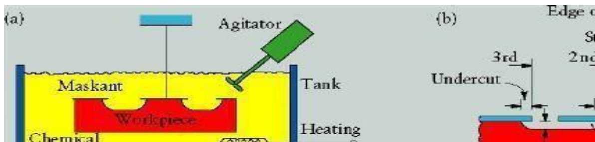
(a) Schematic of chemical machining process (b) Stages in producing a profiled cavity by chemical machining (Kalpakjain & Schmid)
