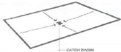
Figure 320-16. Perimeter edge level—slope to center drain inlet.
