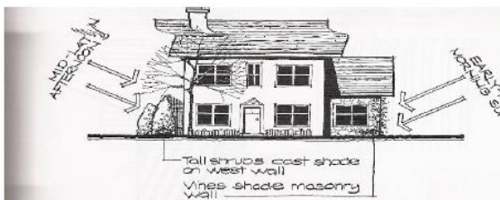
TALL SHRUBS & VINES ON WALLS CAN PROVIDE SHADE FROM THE LOW SUN ANGLE TO THE EAST & WEST.
