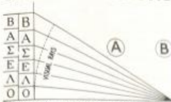
A CORRECTION OF APPARENT PROPORTIONS FROM AN INSCRIPTION ON THE FACES OF THE ANTE OF A TEMPLE AT PRISNE.
