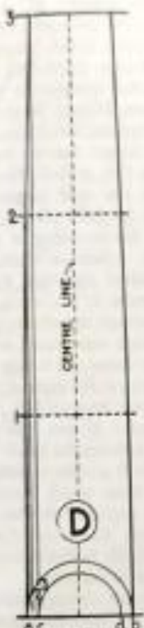
D METHOD FOR ENTASIS a & c ARE BOTTOM + TOP DIAMETERS RESPECTIVELY DESCRIBE SEMICIRCLES ON THESE AT c ERRECT PERPENDICULAR CUTTING LARGER ONE IN 5 DIVIDE SEGMENT a b 3 + HEIGHT OF COLUMN INTO ANY NUMBER OF EQUAL PARTS SAY 5 + NUMBER BOTH 1,2,3 FROM a THIRD POINTS 1,2,3 IN SEGMENT ERRECT PERPENDICULARS CUTTING CORRESPONDING DIVISIONS OF THE HEIGHT THRO THE POINTS THUS OBTAINED DRAW CURVE
