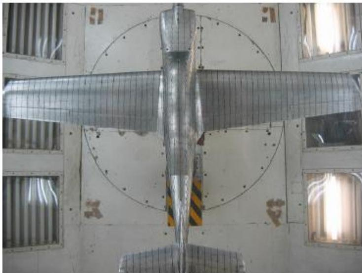
**Figure 5.20.** Flow visualization with cotton tufts in wind tunnel T-35 for flow with  $V = 100 \text{ m/s}$
