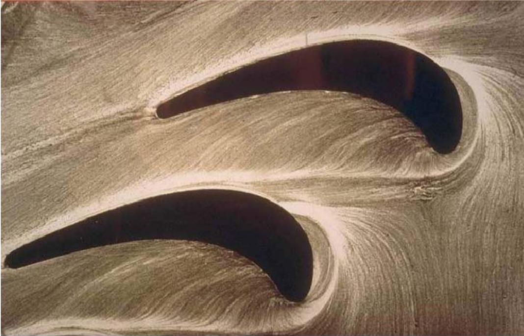
**Figure 5.23.** Oil flow visualization, airflow on the end wall of a turbine blade cascade. (Von Karman Institute)
