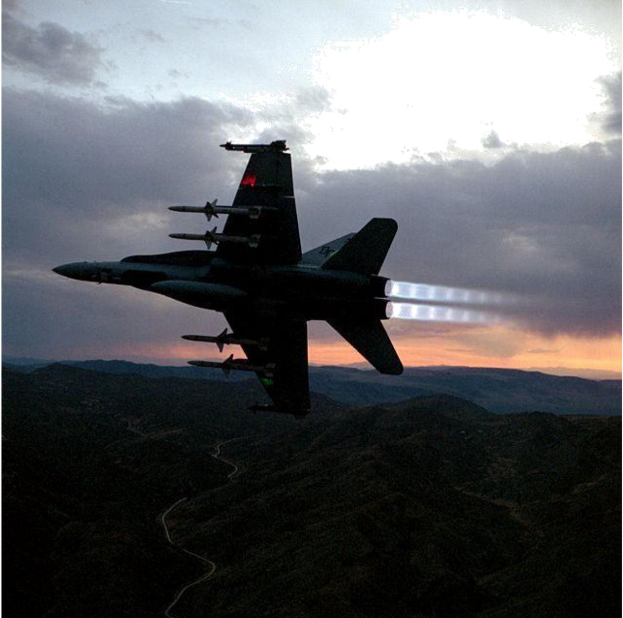
**Fig. 2. 7** A Boeing F/A-18 with afterburners on. Note shock/expansion patterns in the supersonic nozzle exhaust.
