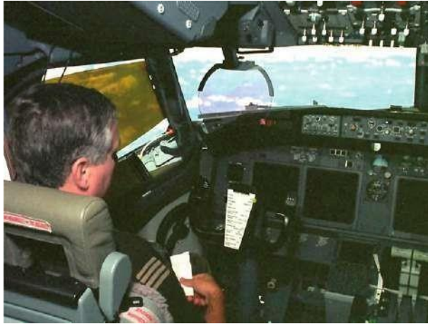
Fig2.3 Civil HUD installation – BAE Systems VGS HUD installed in a Boeing 737-800 series airliner (by courtesy of BAE Systems).
