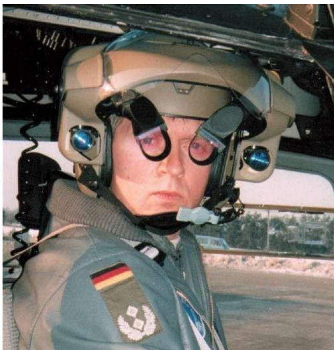
Fig 2.22. Helicopter HMD with integrated NVGs (by courtesy of BAE Systems). This HMD forms part of the mission systems avionics for the Tiger 2 attack helicopter for the German army.
