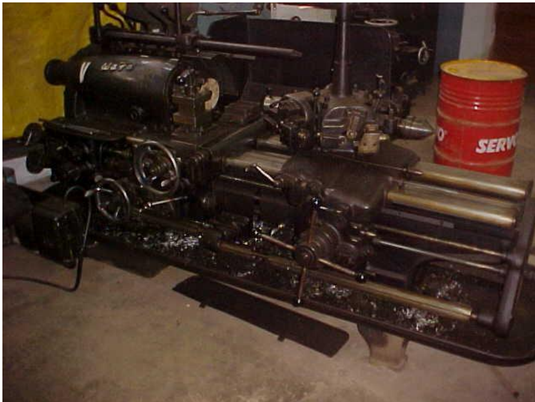
Fig 4 Pictorial view of a turret lathe.
