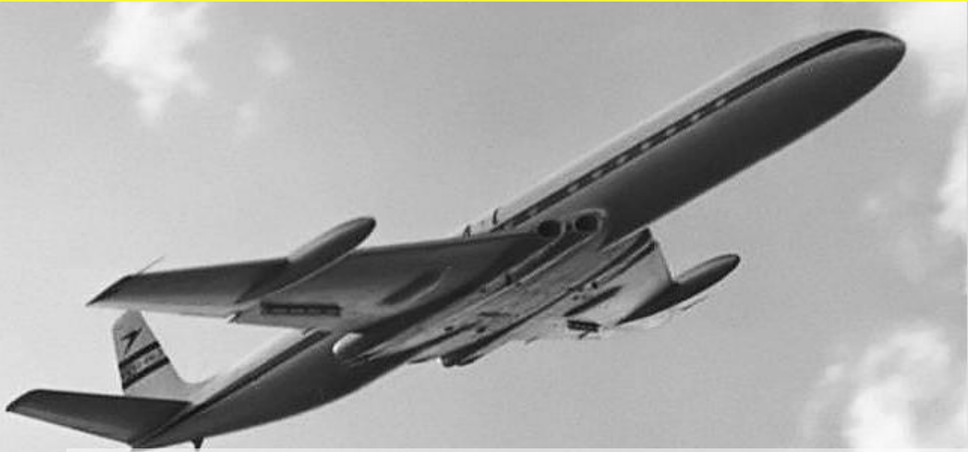
De Havilland DH.106 Comet, Great Britain, 1949 Take-off mass 73.5 ton, wingspan 35 m
