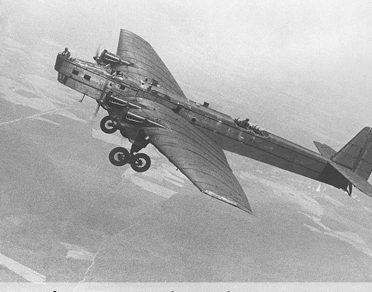
Tupolev TB-3, Soviet Union, 1932 Take-off mass 19 500 kg, wingspan 39.5 m
