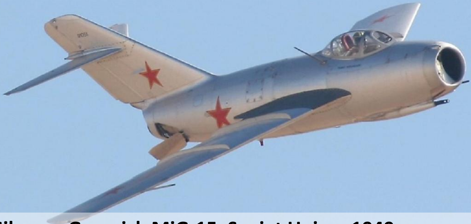
Mikoyan-Gurevich MiG-15, Soviet Union, 1949 Take-off mass 4 917 kg, wingspan 10 m
