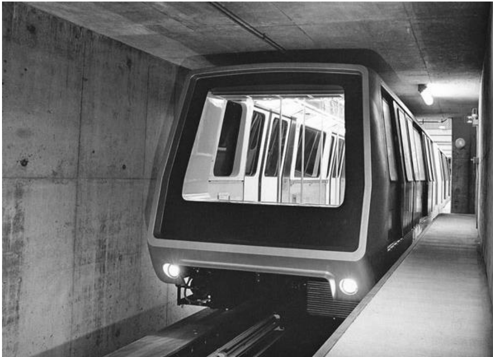
FIGURE 10-17 Automated People Mover (APM) Vehicle at the Greater Pittsburgh International Airport.
