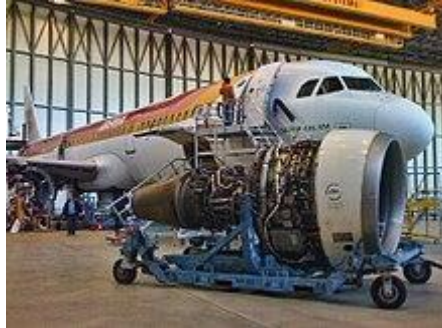
Fig:1.1 An A321 from Iberia having its CFM56 changed
