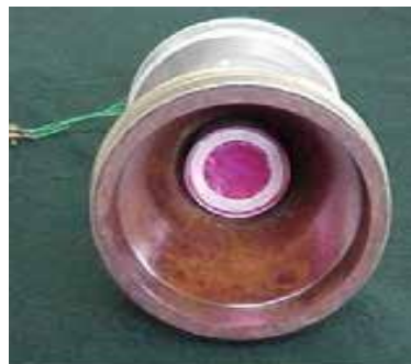
Fig-3: The hot surface igniter
