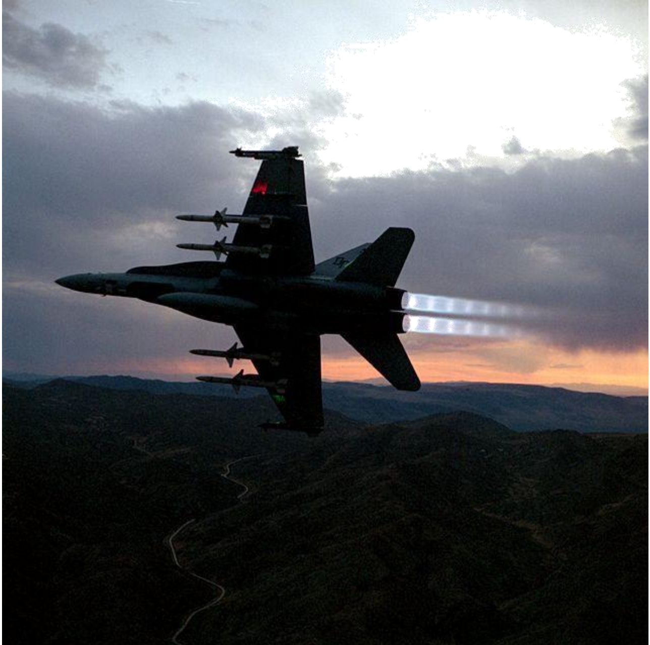
A Boeing F/A-18 with afterburners on. Note shock/expansion patterns in the supersonic nozzle exhaust.
